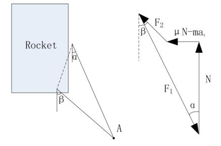
Figure.3 Force analysis of the foot pad
