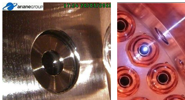
Figure 17: Optical access tube and laser plasma
