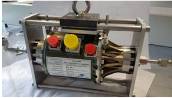
Figure 11: OCV/TCV/RGV demonstrator valve mounted for the cold test campaign (the geometry of the inlet flange is manufactured using an ALM technique)
