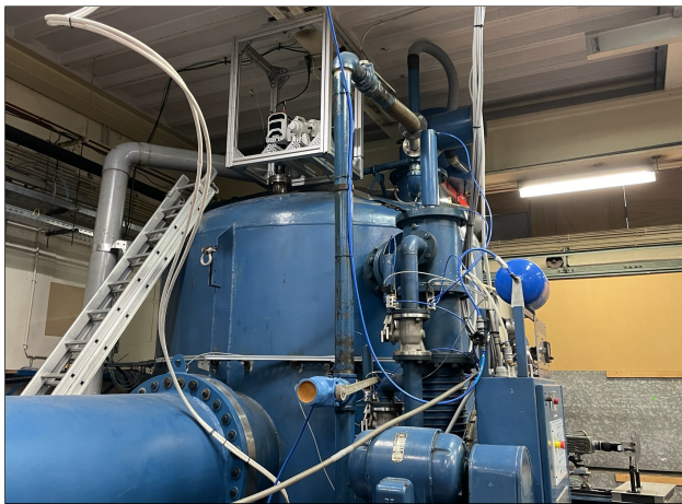
(a) Top view camera positioned above the test section and side view camera facing the mirror of the schlieren system.
