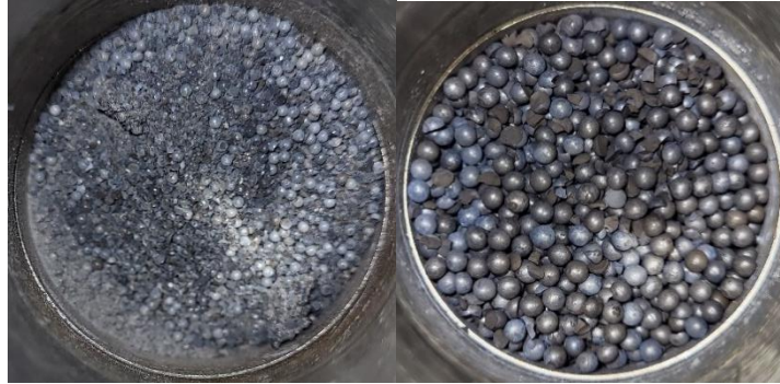
Fig. 8 Visual inspection of the catalyst bed (inlet cross section) physical damage after decomposition 1 kg of HTP 98% for CC_1_1283 (left) and CC_2_1283 (right)
