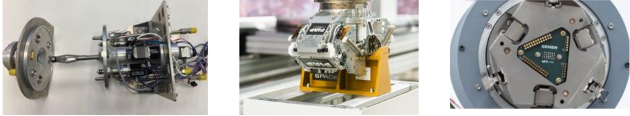
Figure 11: Promising interfaces candidates identified by the Primes, from left to right: ASSIST – GMV, Gripper and Standard Gripping Fixture – PIAP Space and SIROM – SENER
