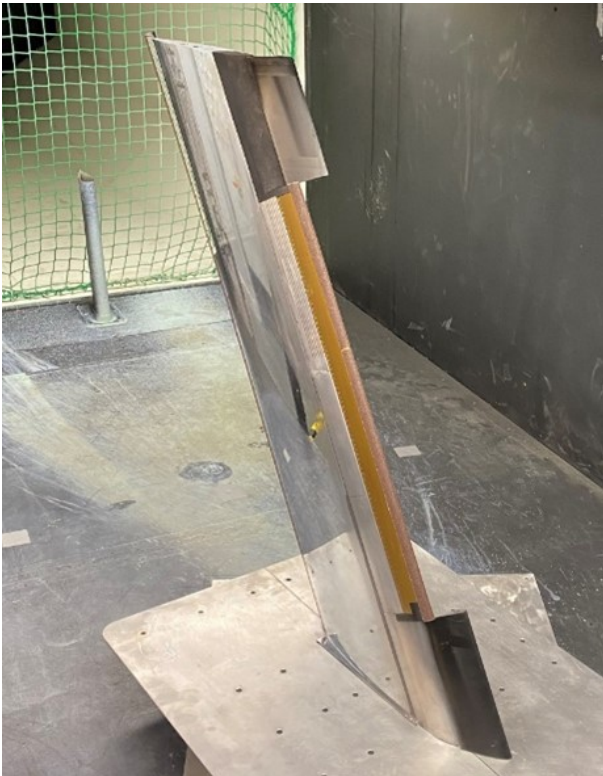
Fig. 3 DLR F-15 model mounted in the wind tunnel.
