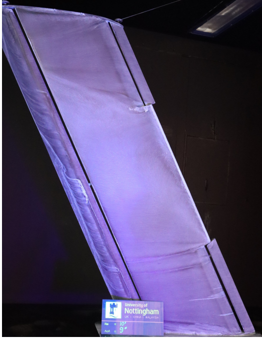
Fig. 5 Oil flow visualisation at \alpha = 9^\circ , starting of the separation at the cut-out. Re=10^6 . (flow from right to left).
