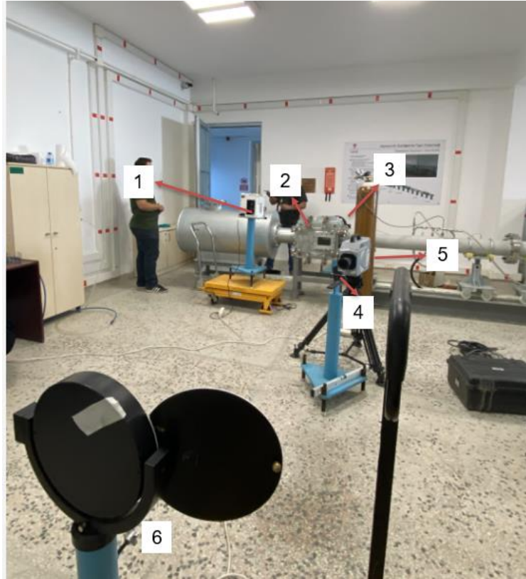
Figure 15: SAGE Expansion Tube Test Facility with schlieren setup (1: Light source, 2: Test section, 3: First parabolic mirror, 4: Knife-edge, 5: Camera, 6: Second parabolic mirror).
