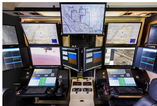
(b) Reaper Block-30 Ground Control Station. Picture from General Atomics Aeronautical Website
