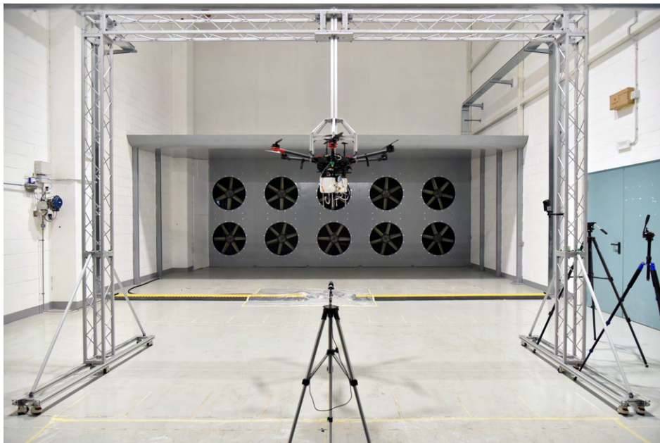
Figure 2: UAS fixed in the SEASTAR Wind Tunnel
