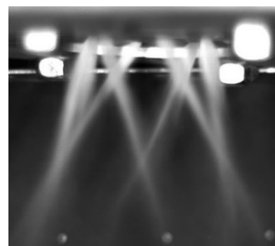
Figure 16. Liquid N_2O discharged through vortex injector
