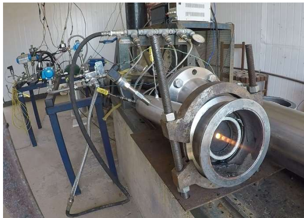
Figure 18. Ramjet test stand with engine operation in nominal regime
