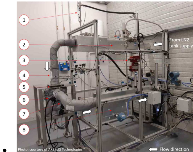
Figure 1: Liquid nitrogen open loop test facility at AREELIS Technologies™ under the thermal insulation blanket. Legend: 1) gaseous helium injection port, 2) inlet Coriolis flowmeter, 3) back-pressure valve, 4) VOF sensor, 5) pump inlet P-T sensors, 6) cryogenic electric centrifugal pump, 7) pump outlet P-T sensors, 8) outlet Coriolis flowmeter.
