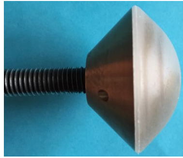
Figure 3: Good-quality subscale Phoebus model obtained using the final sintering procedure.
