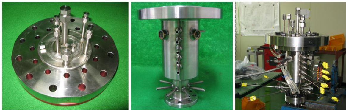
Figure 8: STDM, (left) head assembly, (center) dump cooling combustion chamber, (right) gas generator assembly
