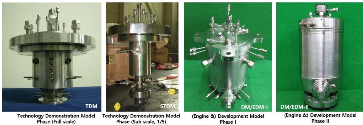
Figure 5: Appearances of the assembled or welded 75 tonf-class gas generators at each phase
