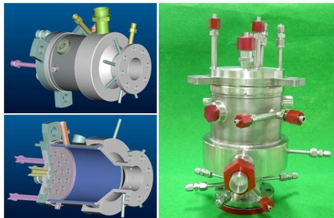
Figure 4: Gas generator developed for the 30 tonf-class open cycle liquid rocket engine
