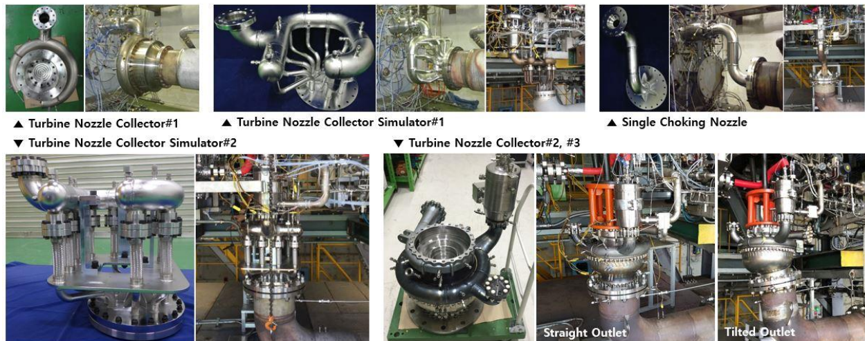
Figure 12: Turbine nozzle collectors, its simulators, and single choking nozzle used in the course of gas generator development test for simulating the actual combustion field
