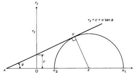
Figure 4: Soil Shear Strength<sup>(3)</sup>.
