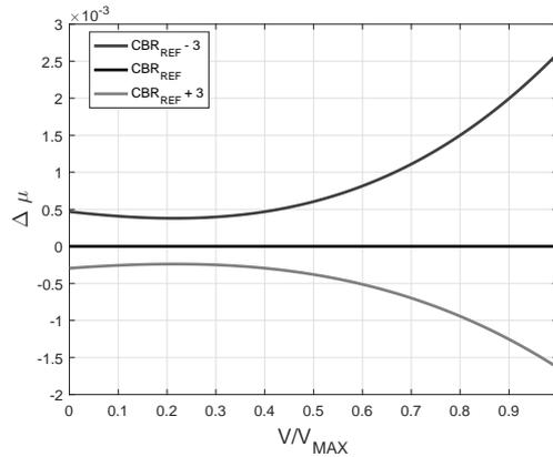
Figure 13: Relation between  $\mu$  and ground speed for soil with vegetation.
