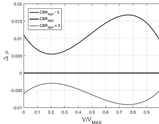
Figure 12: Relation between  $\mu$  and ground speed for soil without vegetation.
