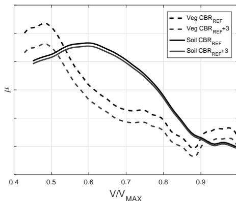
Figure 14: Relation between braked  $\mu$  and ground speed.
