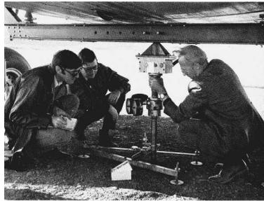
Figure 5: CBR Evaluation for Fokker F28 Certification Tests<sup>(3)</sup>.
