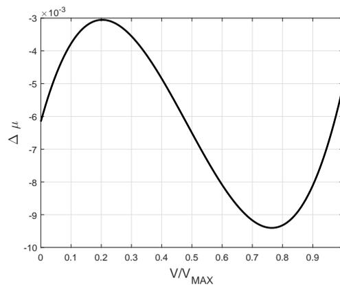
Figure 16: Example of the effect of -30 tons in aircraft weight.
