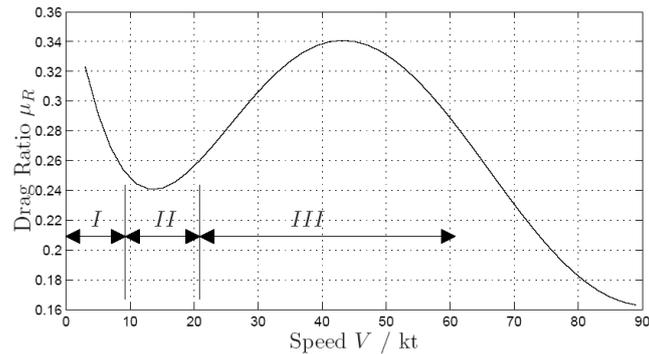
Figure 9: Drag Ratio with speed over unpaved runways<sup>(3)</sup>.
