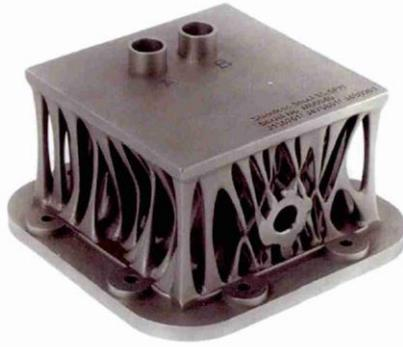
c 3D printed structure with load bearing and heat dissipation
