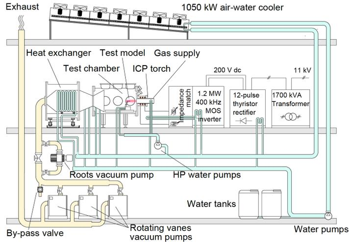
Figure 4: The VKI-Plasmatron facility.
