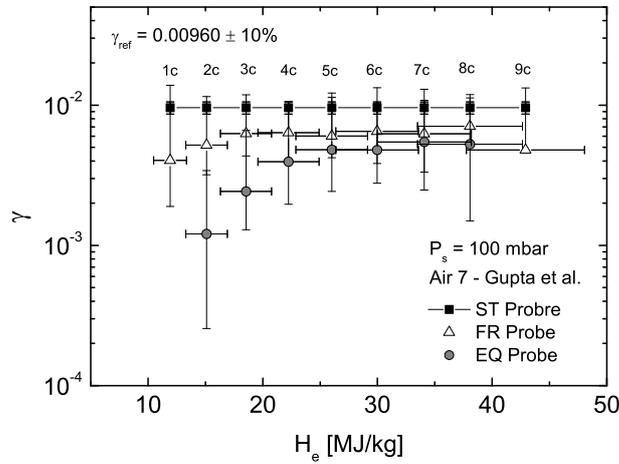
Figure 13: Recombination coefficients on the Damköhler probes at 100 mbar.
