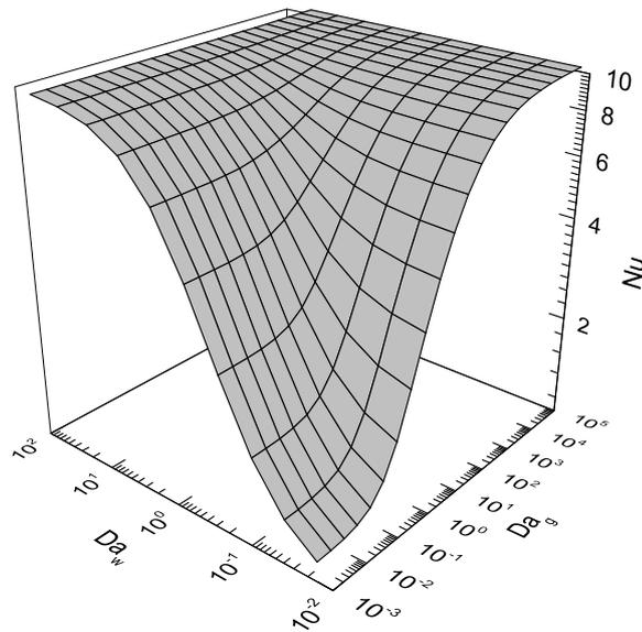
Figure 3:  $Nu$  number as a function of  $Da_g$  and  $Da_w$  for  $H = 9$ , as proposed by Rosner.<sup>15</sup>
