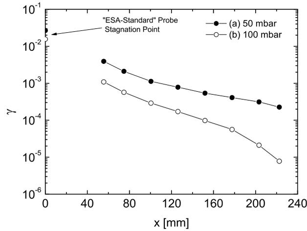
Figure 2: Recombination coefficients on copper determined along a linear calorimeter inserted in a flat plate model.<sup>18</sup>
