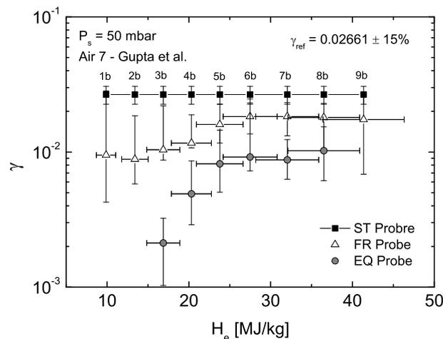
Figure 9: Recombination coefficients on the Damköhler probes at 50 mbar.
