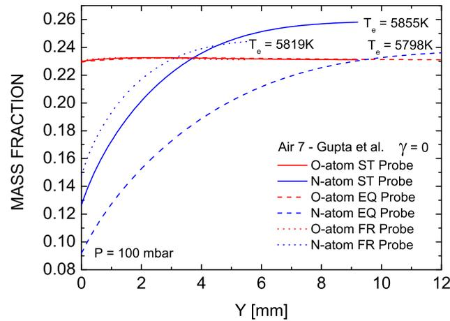
Figure 7: Example of the O and N profiles among the Damköhler probes for the same testing conditions of temperature and pressure and a non-catalytic wall.
