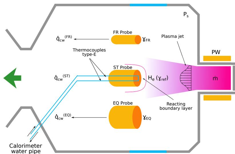
Figure 8: Plasmatron test configuration for catalysis determination on the Damköhler probes.
