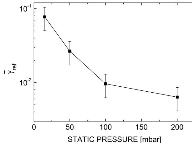
Figure 1: Recombination coefficients on copper calorimeter determined at different pressures in Plasmatron chamber.<sup>17</sup>
