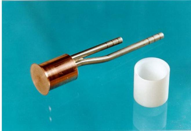
Figure 6: Copper calorimeter inserted in Damköhler probes.
