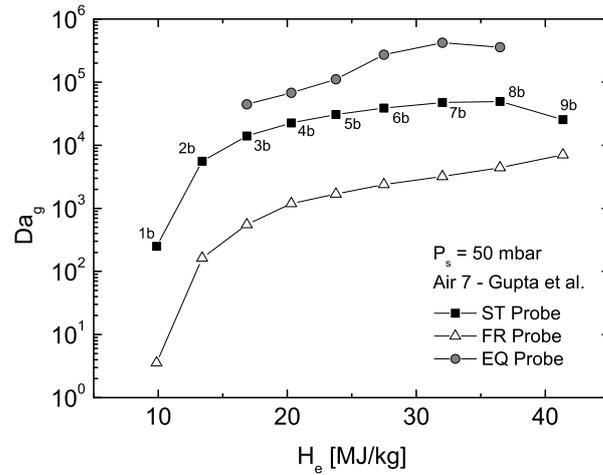
Figure 11:  $Da_g$  on the Damköhler probes at 50 mbar.
