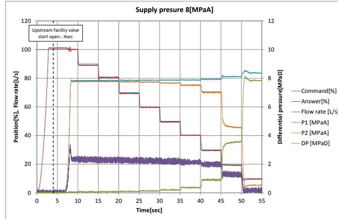
Figure 8: Command / answer history of flow test (supply pressure 8 MPa).
