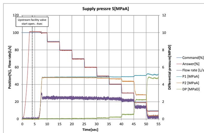
Figure 7: Command / answer history of flow test (supply pressure 5 MPa).
