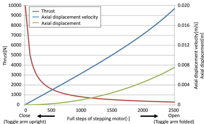
Figure 4: Thrust profile of 3D toggle (example).
