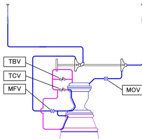
Figure 1: Engine system diagram with nozzle extension
