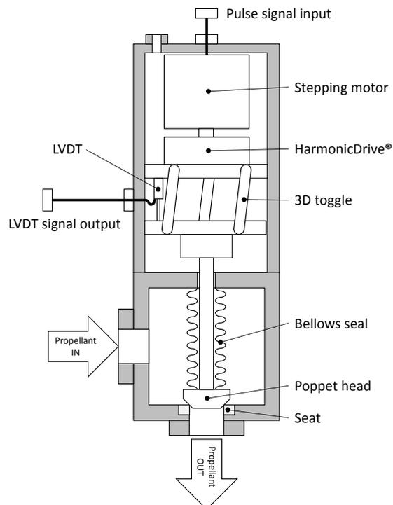
Figure 2: Valve configuration.
