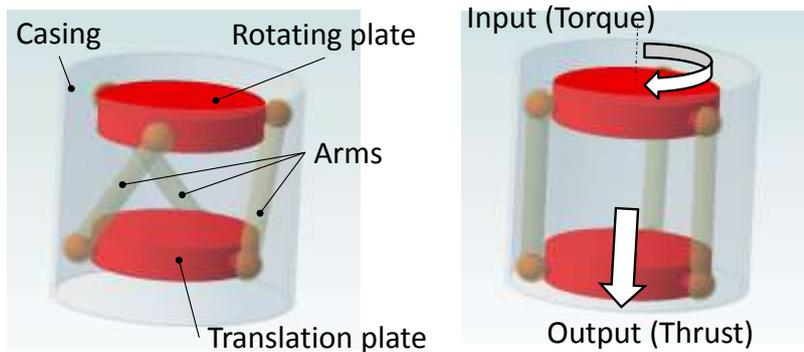
Figure 3: 3D toggle configuration.
