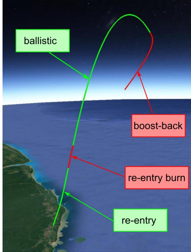
Figure 1: Return trajectory for the Toss Back concept
