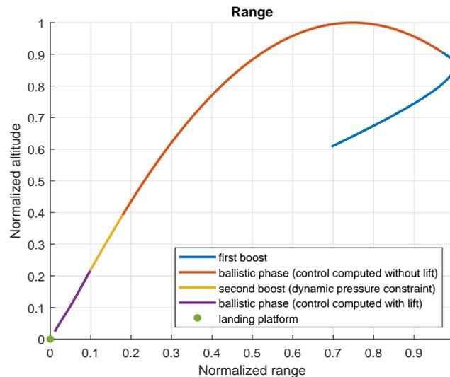
Figure 2: Altitude of the vehicle in function of its range to the landing platform
