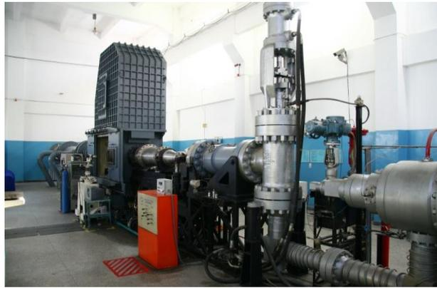
Figure 1: The FD-07 hypersonic wind tunnel
