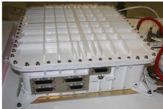
Figure 2. Main Electronics unit of IMaX before the integration
