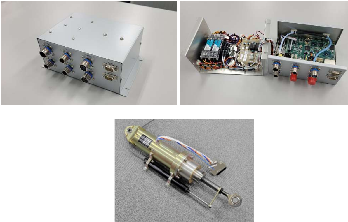
Figure 12 : Thrust Vector Control (TVC) controller (top) and actuator (down)
