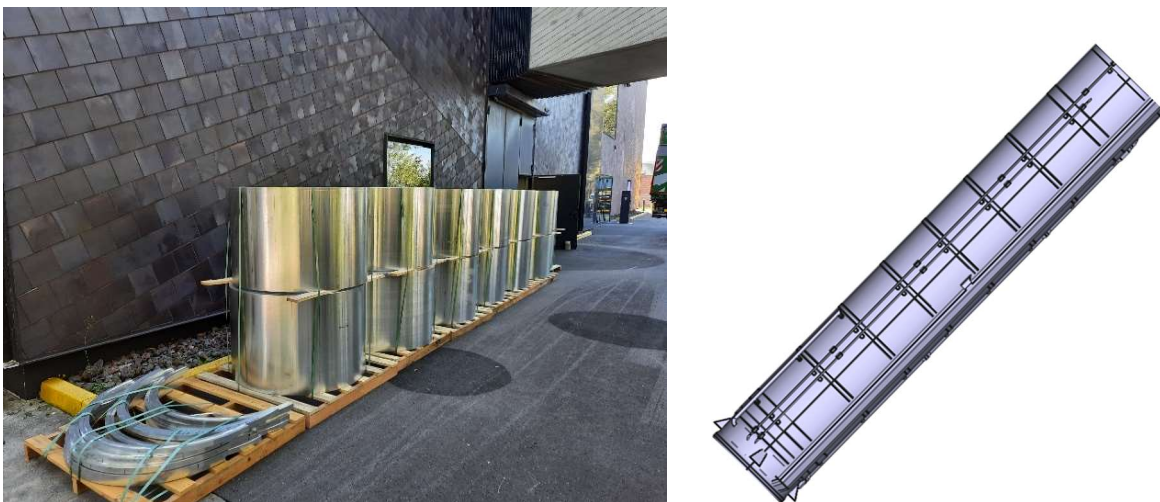
Figure 6 : Propellant tanks H/W (left) / Overall Design (right)
