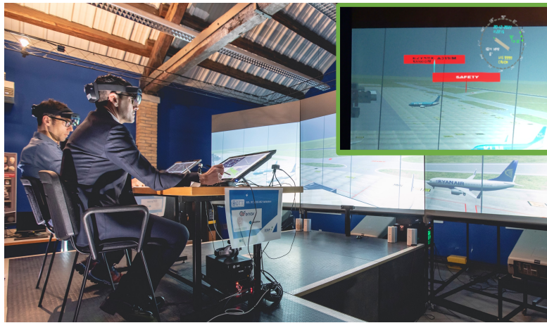
Figure 2: The ATCOs can contemporarily see both the out-of-the-tower view and the Augmented Reality Overlays through HoloLens2. The personal view of the user during the XR Safety Net validation exercise is depicted in the green square.
