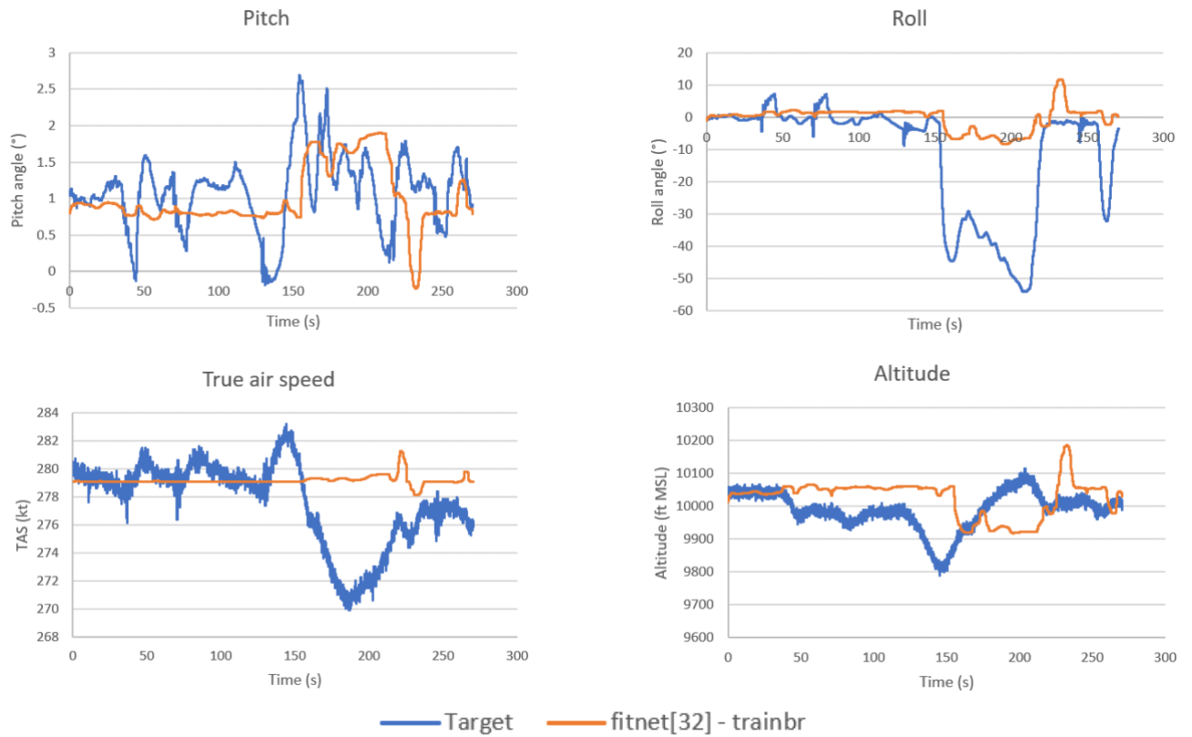
Figure 5: Predictions for Rudder Doublet 240 kt manoeuvre with one trained manoeuvre
