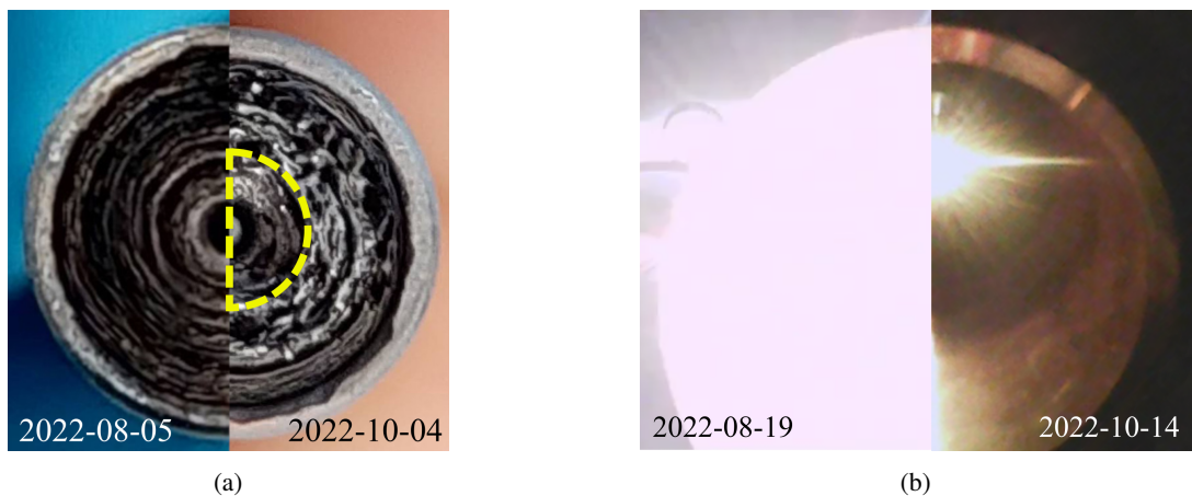
Figure 5: Comparisons exhibiting degradation to the tantalum-emitter cathode over time. (a) picture of the cathode tip at installation. After two months of operation a significant amount of mass has been lost in the region marked in dashed yellow lines. (b) picture of the plasma produced by the cathode under identical operating conditions (1.8 A keeper current, 0.5 mg/s argon flow, 1.3 mm keeper orifice) approximately two months apart, with the picture on the left side being saturated due to light emission from the cathode. Pictures are taken looking directly towards the tip of the cathode. Note that in both cases the anode is in place, but is not energized.
