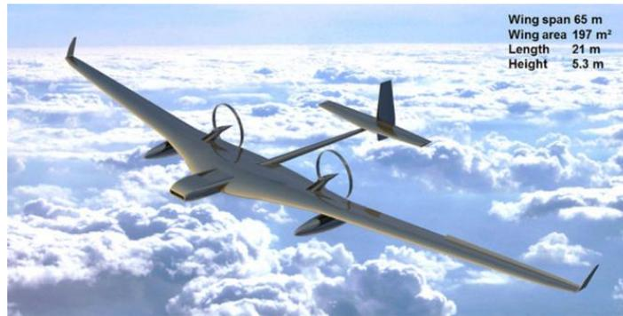
Figure 1-1: “StratoStreamer” HAPS aircraft [11]
