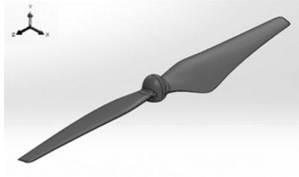
Figure 1- DJI-9450 single- rotor configuration CAD
