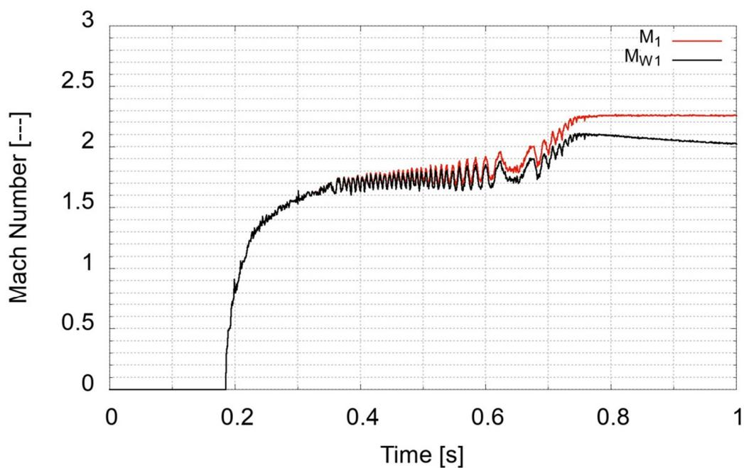
Figure 5: Stator Mach number at outlet and Rotor relative inlet Mach number
