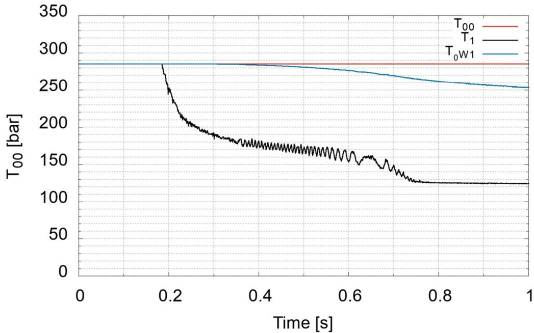
Figure 4: Total inlet and static outlet Temperature at stator and total inlet temperature at stator in relative rotating frame
