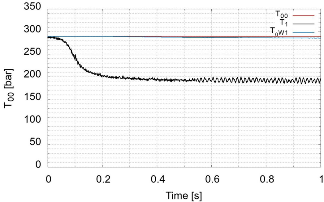
Figure 9: Total inlet and static outlet Temperature at stator and total inlet temperature at stator in relative rotating frame
