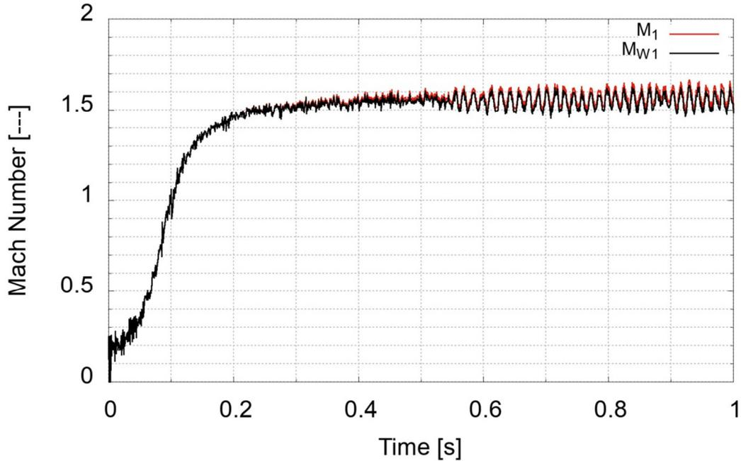
Figure 10: Stator Mach number at outlet and Rotor relative inlet Mach Number
