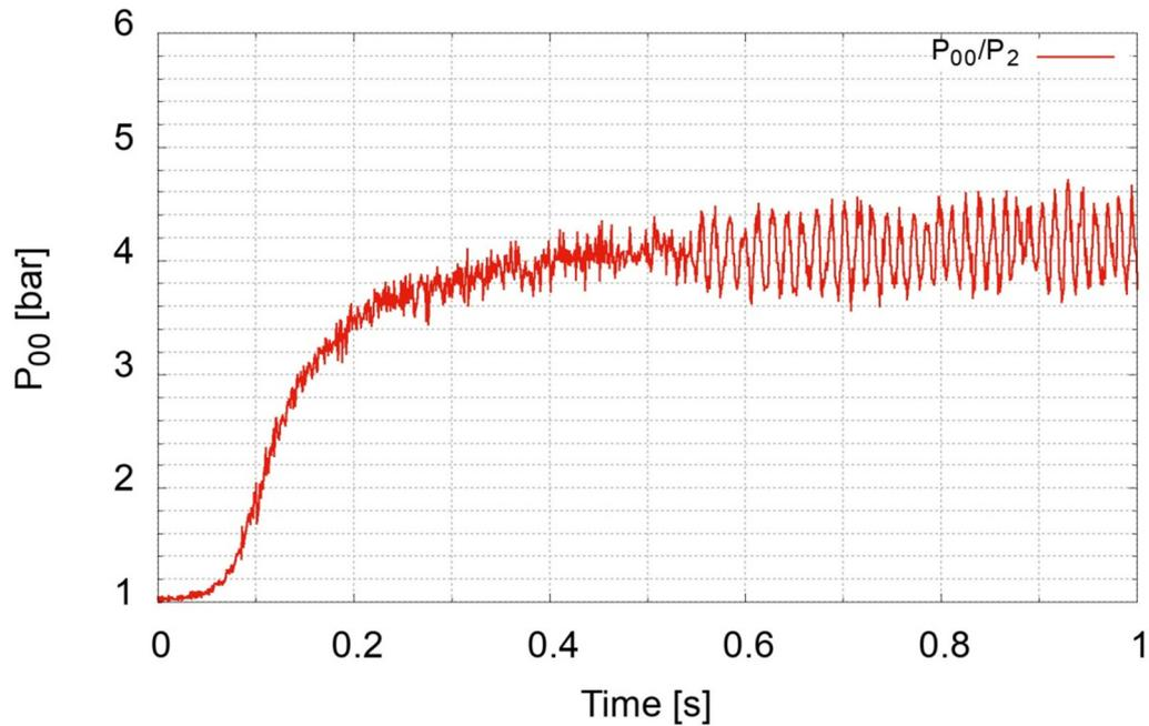
Figure 7: Stator pressure ratio (Total-to-static)
