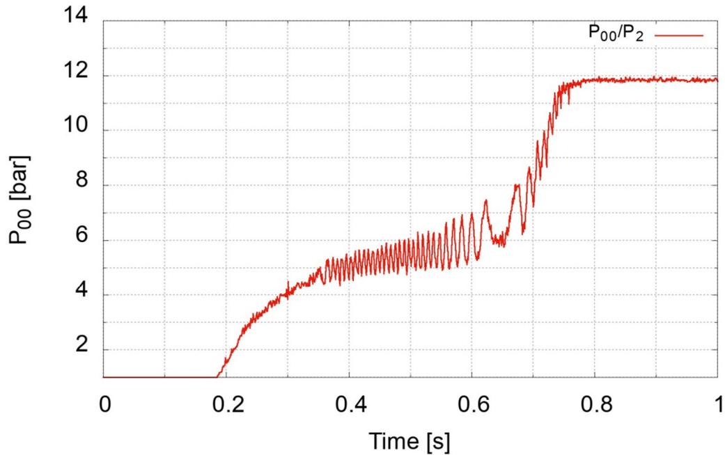
Figure 2: Stator pressure ratio (Total-to-static)
