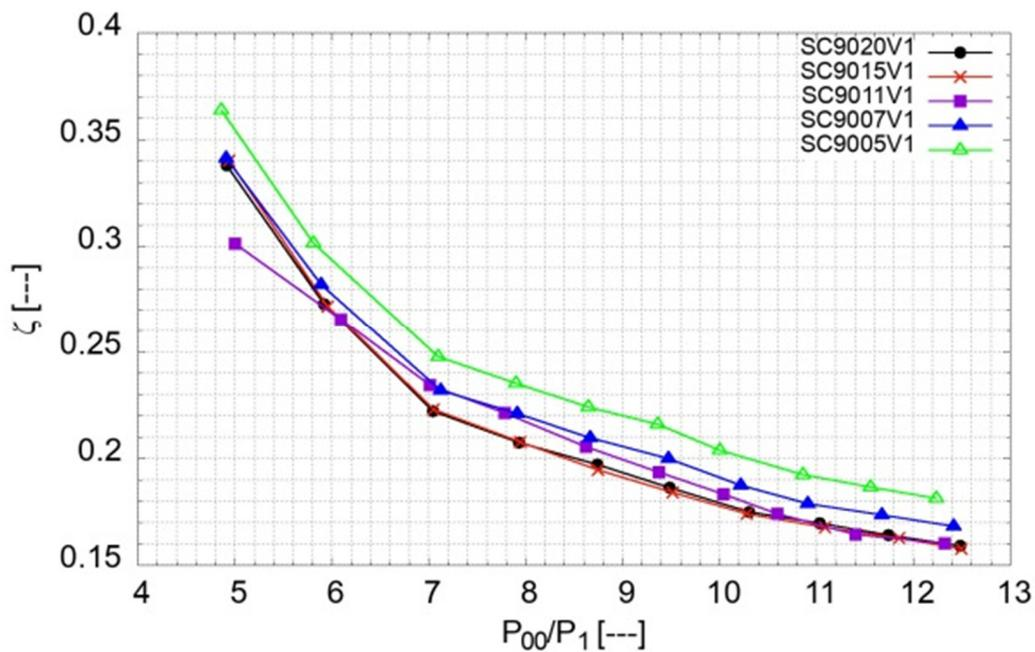
Figure 11: Stator losses in function of outlet Mach number for various profiles [ 9
