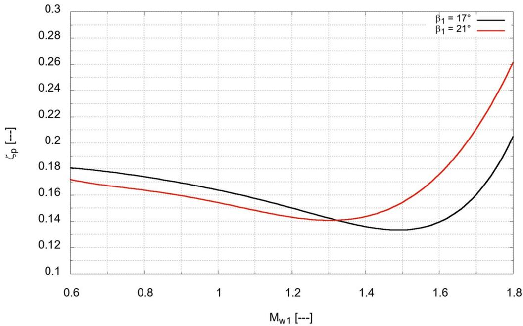
Figure 12: Rotor losses in function of Inlet Mach number
