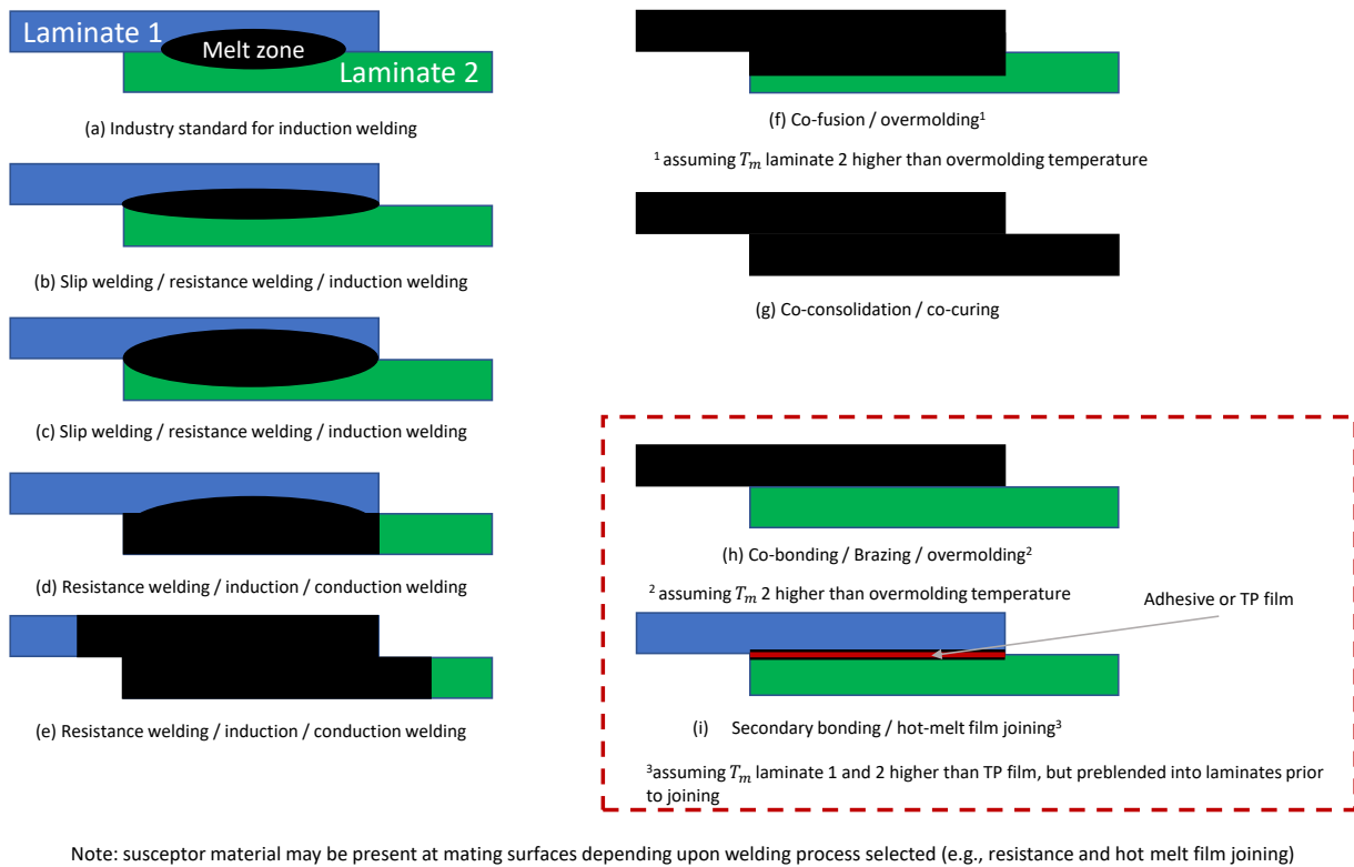
Figure 1: Overview of welding technologies (classified by the size of the weld pool)
