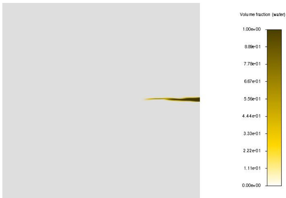
Figure 2: Liquid jet after 0.05ms after the onset of the injection. The instability arises clearly and leads to a elongation of the liquid jet.
