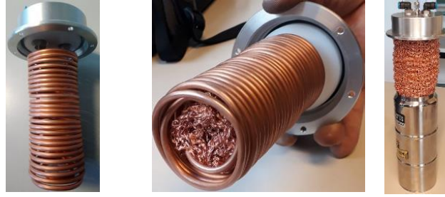
Figure 8: FLORENCE HEX design including a vacuum-insulated thermos, a copper serpentine, an aluminum lid, a thermocouple feedthrough, and a copper mesh.
