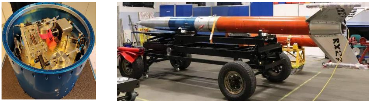
Figure 5: FLORENCE experiment module (left) and the integrated REXUS-27 rocket (right).
