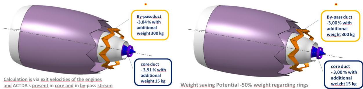
Figure 23: Fuel saving potential for thrust generation under ideal conditions (left) and under estimated real conditions (right) for thrust generated in the core/ and in the bypass stream. The total potential under real condition can be figured out with help of the thrust ratio in cruise between core and bypass stream, and is for an SA-aircraft exemplary engine set of two engines 3% fuel savings for the aircraft in cruise flight, with components efficiency of thrust crowns, estimated, being 78%
