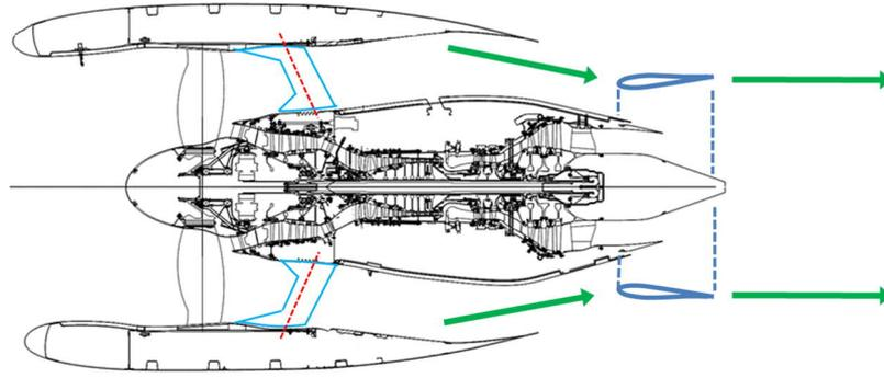
Figure 16: Correction of the conical thrust displacement by a ring-shaped wing (named Thrust Crown, TC), exemplary shown in the bypass-duct. The TC deviates/corrects the exit velocity in/to flight direction. The ring (TC) acts like a teeth-retainer for the engine
