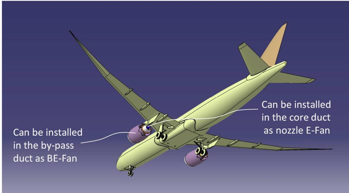
Figure 22: Possibilities to install E-Fan and/or Thrust Crowns in the engines of an aircraft. Core E-Fan and Thrust Crowns in general can be retrofitted to existing/ in production engines an aircraft, also including wide body aircraft
