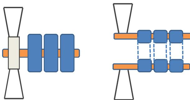
Figure 12: Two possibilities in principal to stack electric motors to add up their power output on same rotational speed on at least one output shaft e.g. for driving a fan, on the left for in-runner electric motors, on the right for out-runner electrical motors mot.
