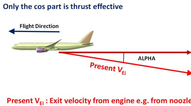
Figure 20 Only the cos-part of the thrust vector with exit velocity becomes thrust effective (effect exaggerated for clarity)
