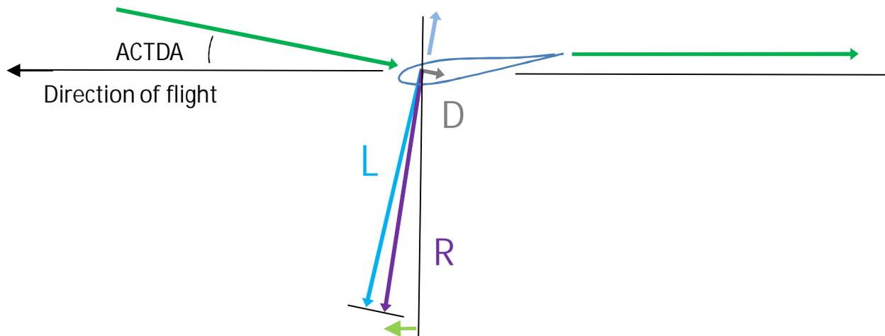
Figure 17: By this arrangement a resulting fluid force at the ring-shaped wing is generated, which is tilted to the front .in flight direction, thus having a propulsive - or drag weakening force on the aircraft, like a winglet
