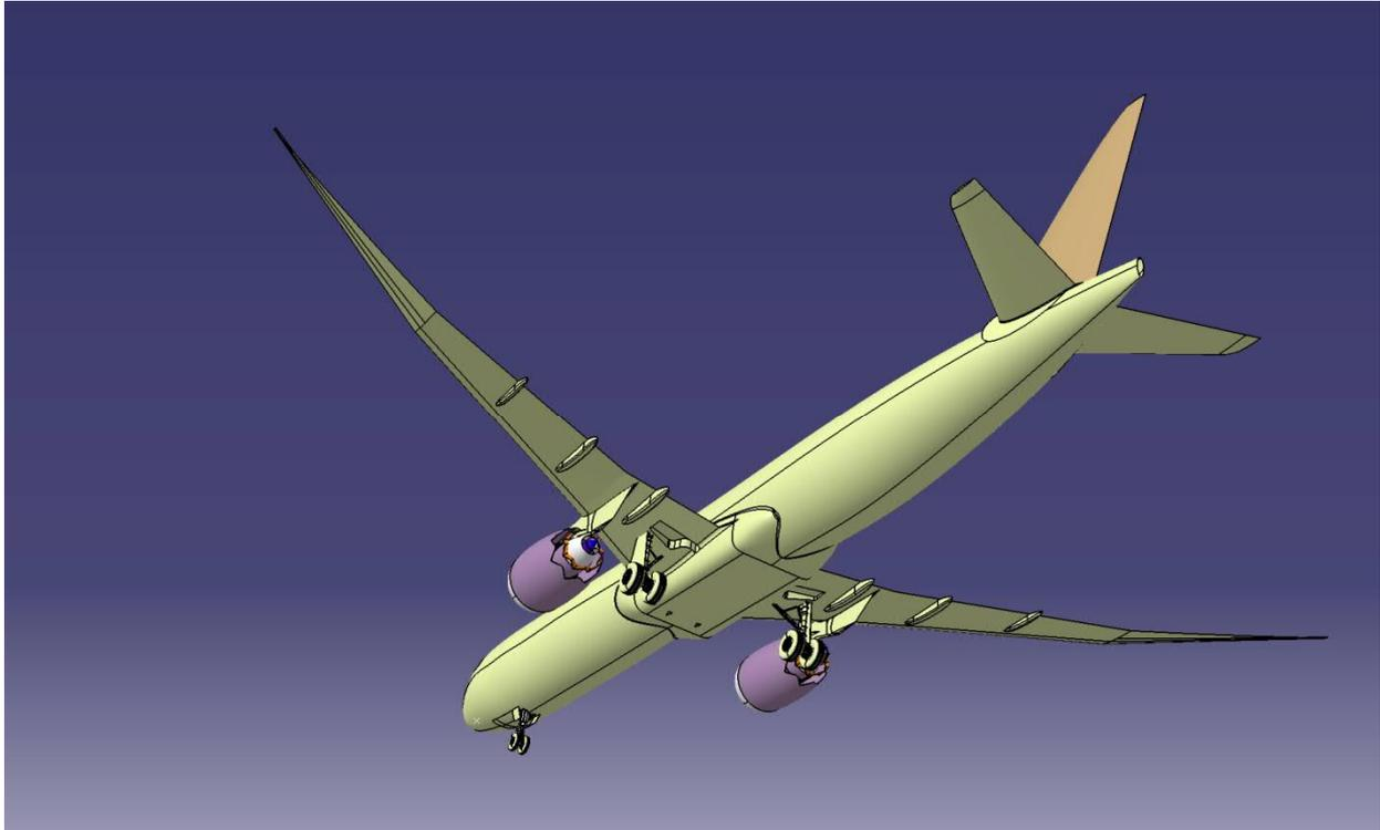
Figure 31: By the increased wing area it gets possible to climb in higher initial and maximum cruising altitudes with less air density and lower drag, thus more fuel efficiency
