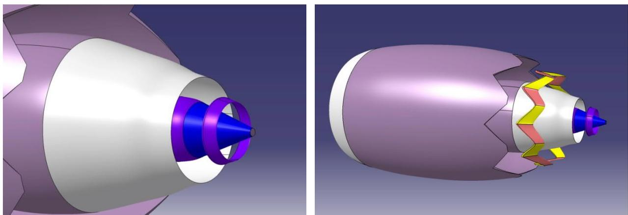
Figure 21: Exemplary embodiments of Thrust Crowns in the core duct (left) an in the by-pass duct (right). In the by-pass duct the ring-shaped wing has to be designed with swept.
