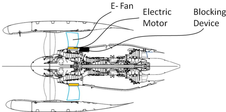
Figure 13: E-Fan integrated in the by-pass duct. This solution allows higher degrees of electrical thrust (degree of hybridization) up to 35% of the by-pass duct thrust, but this of course it leads to higher additional weight regarding installation and electrical storage. But it can be also just used in special flight stages e.g. during climb (out)
