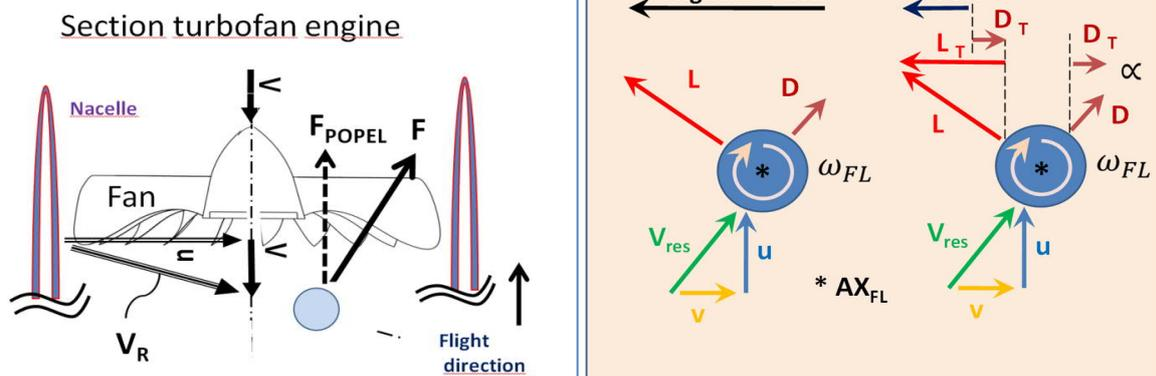
Figure 3: Forward facing Propulsive Force generated by flettners as active (elect.) stator device downstream of a fan
