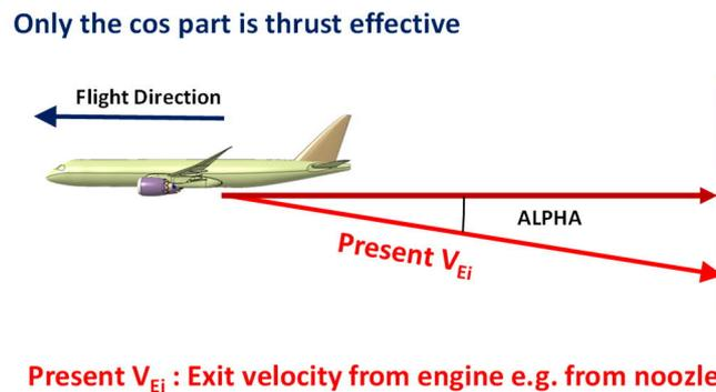
Figure 14 : Only the cos-part regarding the angle alpha of - the thrust vector, formed by exit velocity  $V_{EI}$  - becomes thrust effective (effect exaggerated for clarity)
