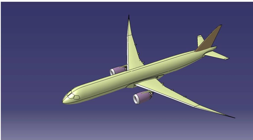
Figure 28: Bearbas 123 XXLR with modified wing ans Thrust Crowns at engines
