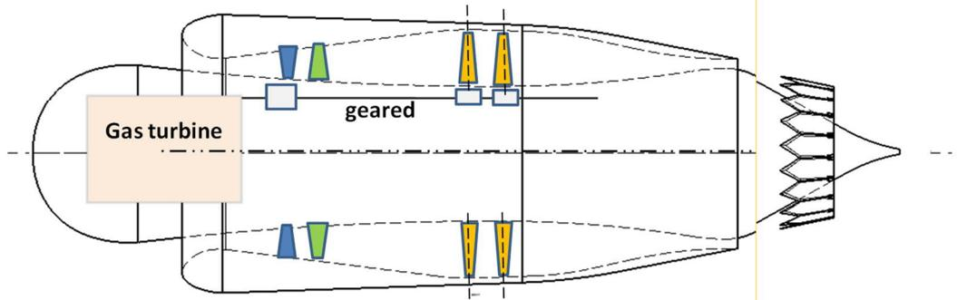
Figure 6: Aircraft engines for higher incoming speeds would need special diffuser means to slow down incoming speed, here two diffusers shown, one open in the inlet area, and one circular over the perimeter, ducted. The fan could be in front or as an aft fan, exemplary engine.
