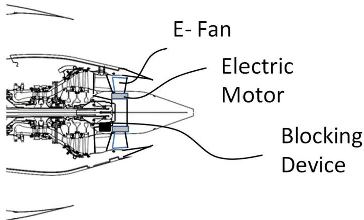
Figure 9 : Detail view of the nozzle E-Fan, - as the conical rear part plug is almost completely empty, there is more than enough room for the integration of electric-motors, furthermore it is placed in flight direction rear of - the mounting or strut connection, which means, that devices can be easily accessed from the behind in operation, if needed, therefore the core E-Fan is in principle been retrofit-able to existing and in production engines and aircraft
