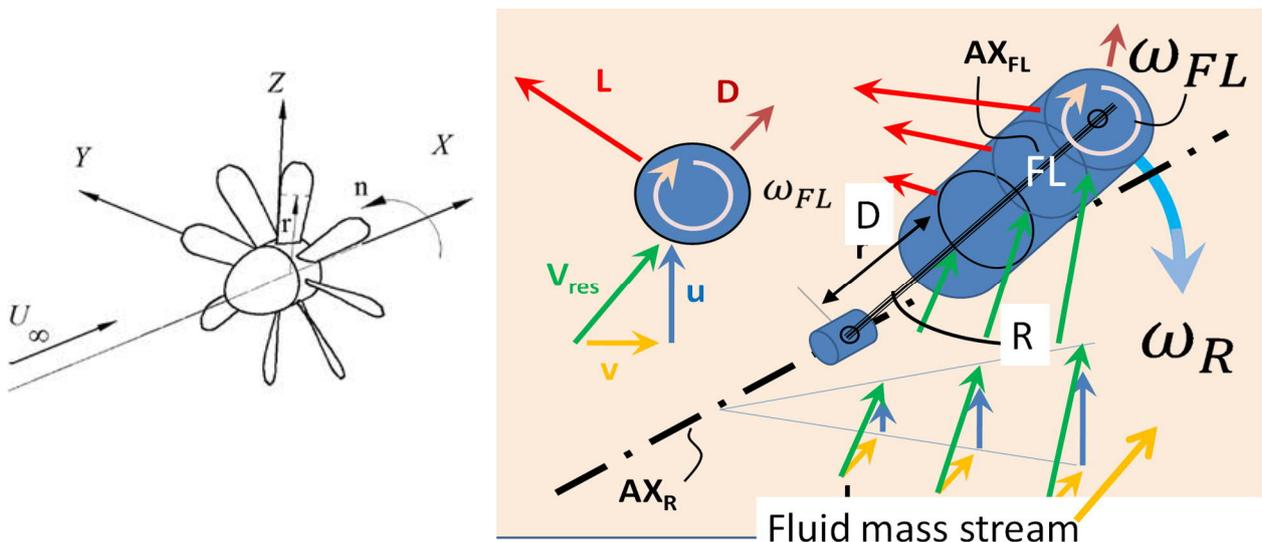
Figure 4 and 5: Flettner rotors, implemented on rotors. They can be electrically driven and controlled. As well they could be placed in a ducted environment, where incoming velocity speed can be controlled, also by means of diffusers
