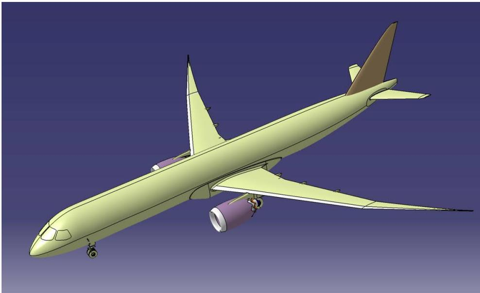
Figure 27: Bearbas 123 XXLR features wing area increase by wing tip devices in “raked wing tip manner” by +10 % whereby they at the same time lower significantly induced drag, thus generating lower overall drag in cruise flight, whereby the increased wing area enables higher cruising altitudes with lower fuel burn
