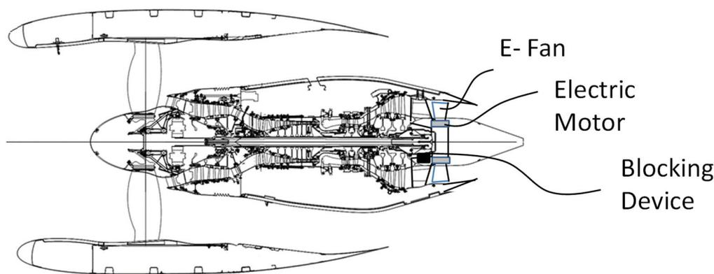
Figure 8: Nozzle E-Fan, integrated in the core stream, upstream the nozzle
