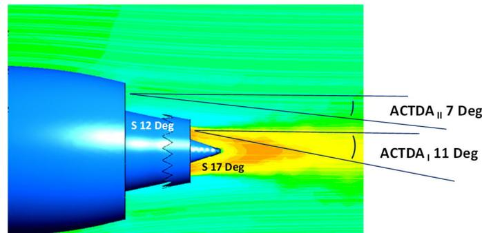
Figure 19 : Average Conical Thrust Displacement Angle (ACTDA) in the core and in the bypass stream and slope angle of the contour (S) at an exemplary engine in cruise flight, the streamlines when leaving the engine parts by exit speed  $v_{Ei}$  are not in line with the flight direction, thus they are angular 3 D displaced
