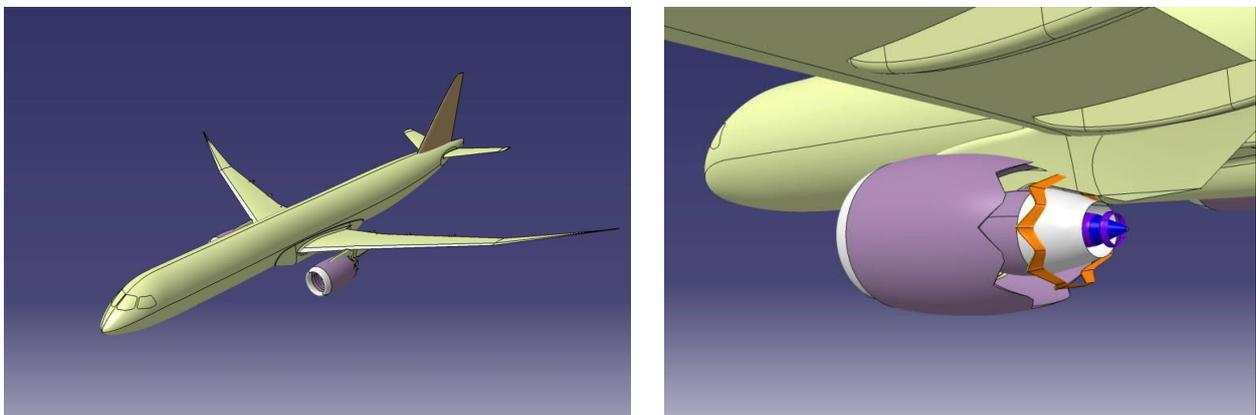
Figure 2 , 30: Bearbas 123 XXL with modified wing in raked-tiü manner and Thrust Crowns installed at engines
