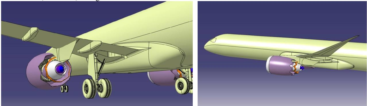
Figure 24 : The thrust crowns (TC) can be fixed to the pylon, as well as additionally to the struts, which links the nacelle to the core engines (here not shown). This applies specifically to the TC in the by-pass area. In the core stream the TC can be fixed to at least one of the nozzle components, preferably to the core engine nozzle e.g. by struts.
