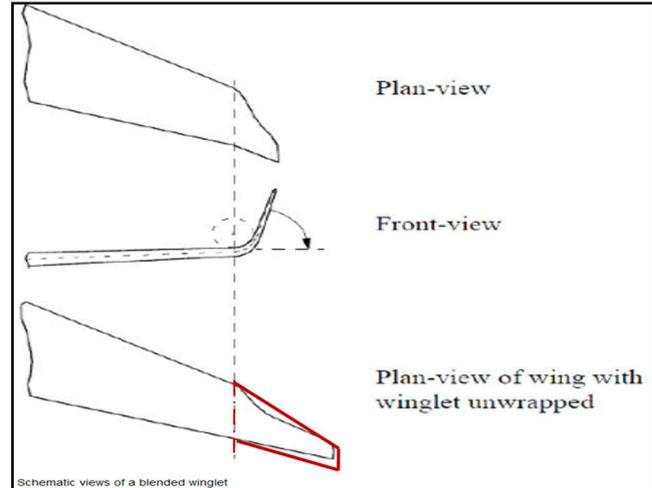
Figure 33: Span extension in a “raked-wing tip” manner leads to a significantly enlarged wing area in contrast to winglets, which are bended up, whereby first helps to boost significantly long range (fuel) performance
