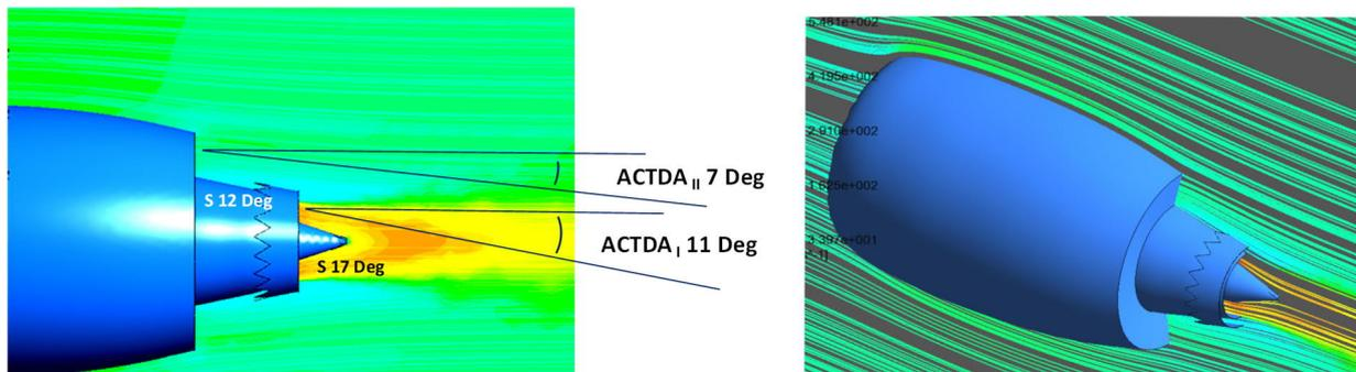
Figure 15 : Average Conical Thrust Displacement Angle (ACTDA) in the core and in the bypass stream and slope angle of the contour (S) at an exemplary engine in cruise flight, the streamlines when leaving the engine parts by exit speed  $V_{EI}$  are not in line with the flight direction, thus they are angular 3 D displaced
