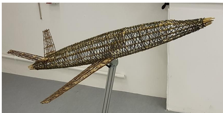
Figure 10. Natural material composite geodesic WrapToR airliner demonstrator
