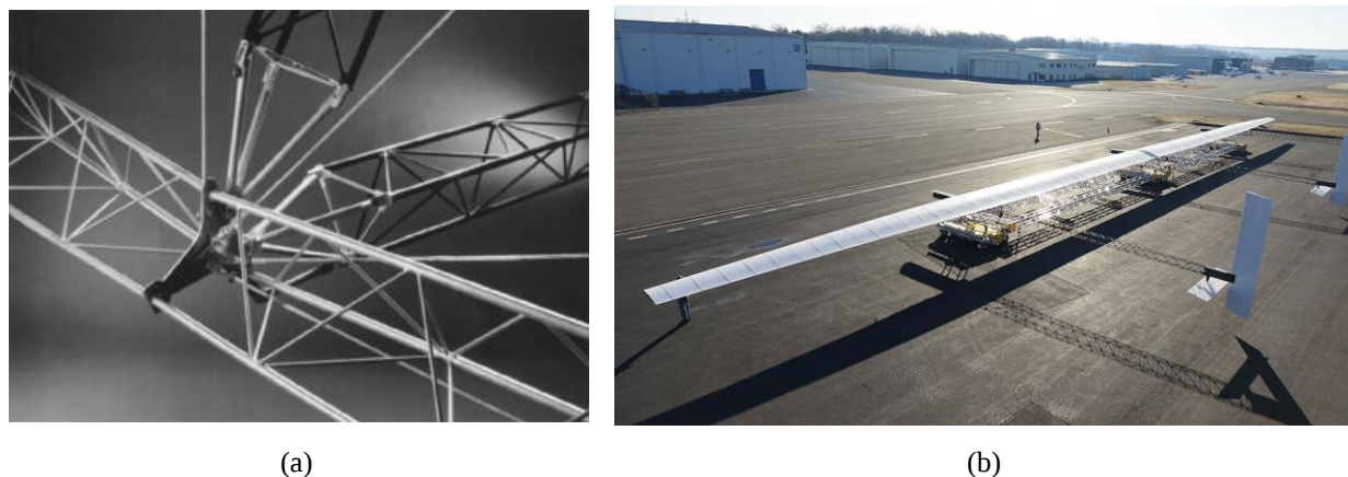
Figure 1. Assembled composite truss structures: a) composite truss beams (in black) within a hybrid material hierarchical space frame on the Zepplin NT [3] and b) truss beams visible in the tail booms of the Aurora Flight Sciences Odyssey high altitude pseudo-satellite [4].
