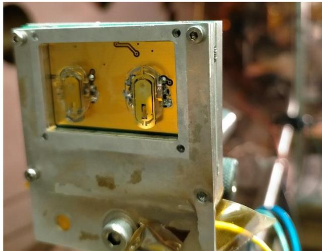
Figure 3: Two sensors mounted on the PCB card. This card is golded to be conductor. The PCB is placed inside the shielded boxes. The whole setup is hold by a translation stage behind (blurred here)
