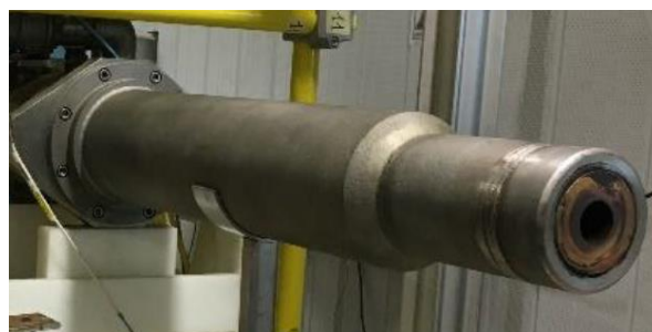
Figure 1 : Arc heated air plasma generator
