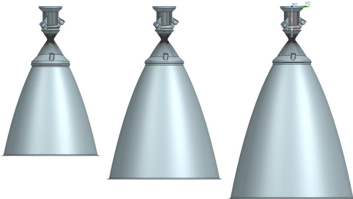
Figure 8: Comparison of RELIANCE nozzle options (from left to right: 1, 2 and 3) side view
