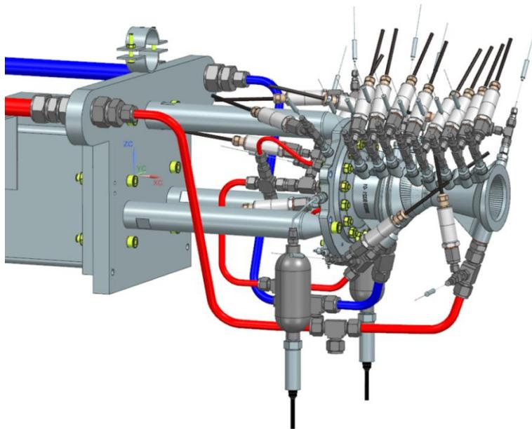
Figure 5: View of the Breadboard Engine CAD Model attached to the Test Stand [9]
