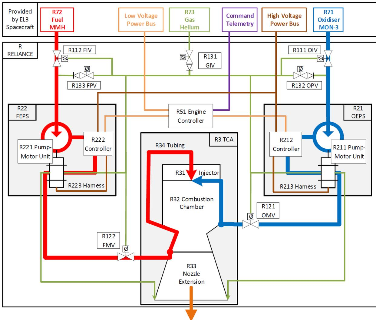
Figure 6: RELIANCE engine system schematic
