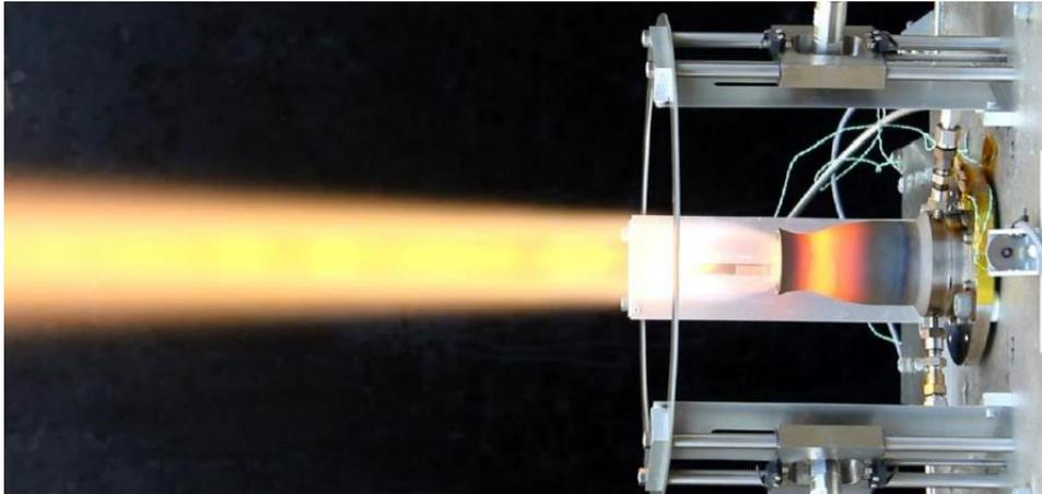
Figure 4: 1.1kN MMH/MON subscale test engine being hot fire tested at sea level in Westcott, UK
