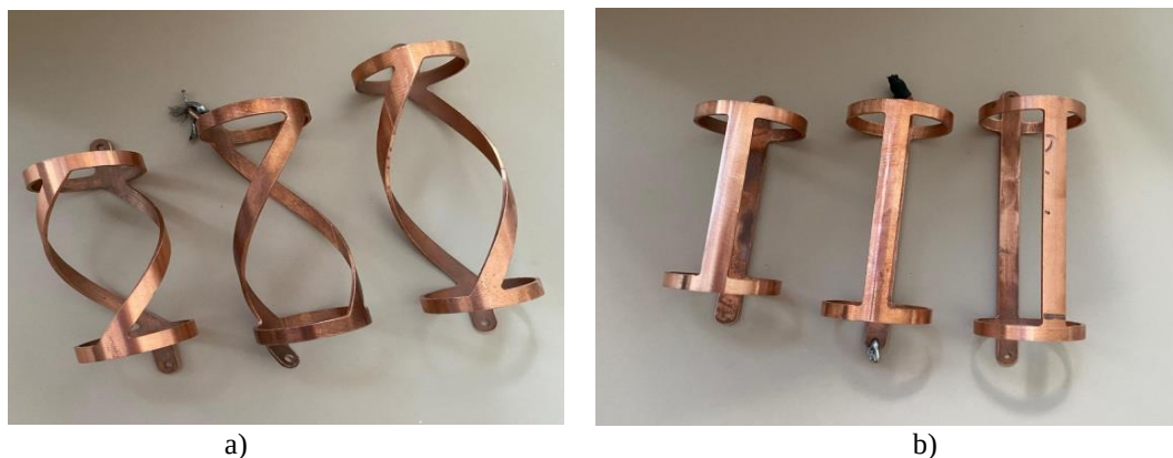
Figure 3: a) Half –wavelength Right Helical Antenna of 65mm, 78mm and 87mm, b) Nagoya Type III Antenna of 65mm, 78mm and 87mm
