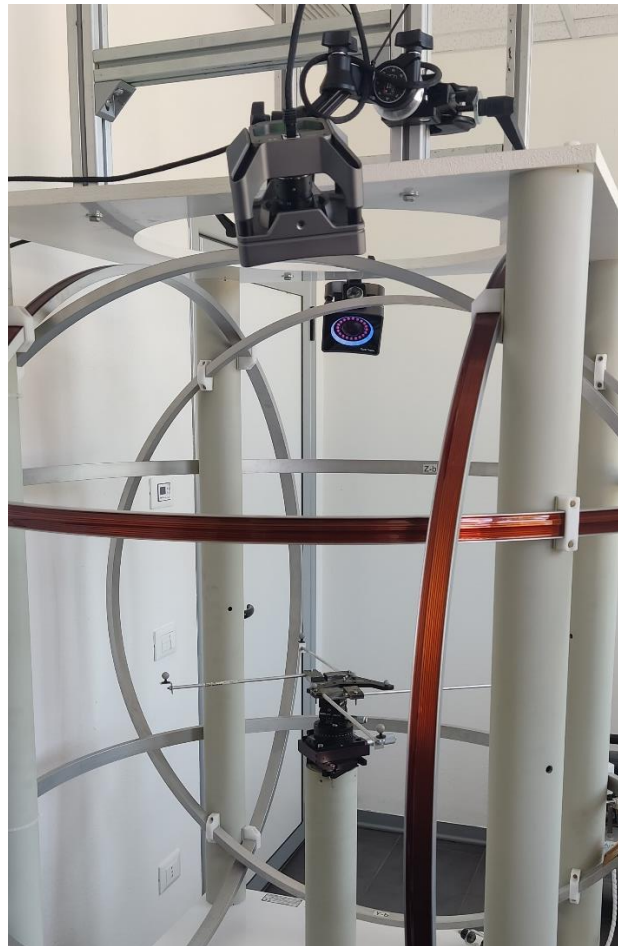
Figure 4: Test set-up for the ground-truth vision system prototype.
