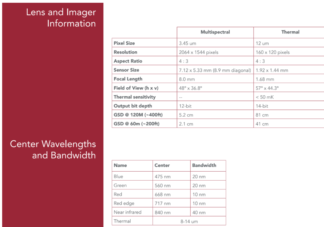
Figure 2 - Micasense Altum technical specs.
