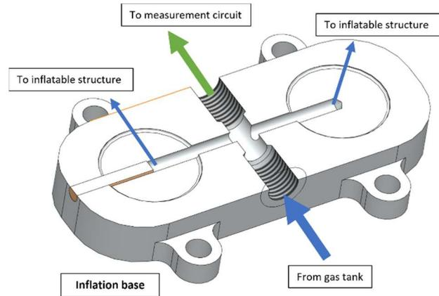
Figure 7: Inflatable structure base (cross-section)
