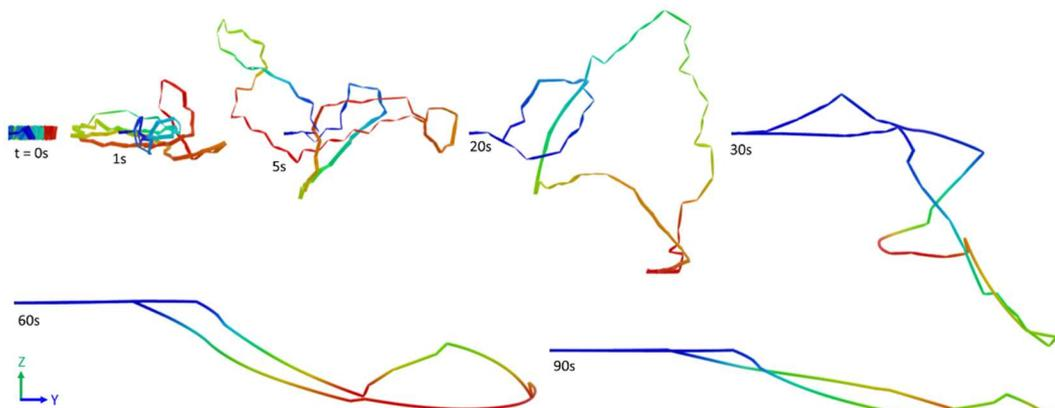
Figure 11: Deployment kinematics of the inflatable structure in the YZ coordinates
