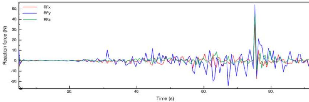
Figure 13: Reaction force components on the platform satellite
