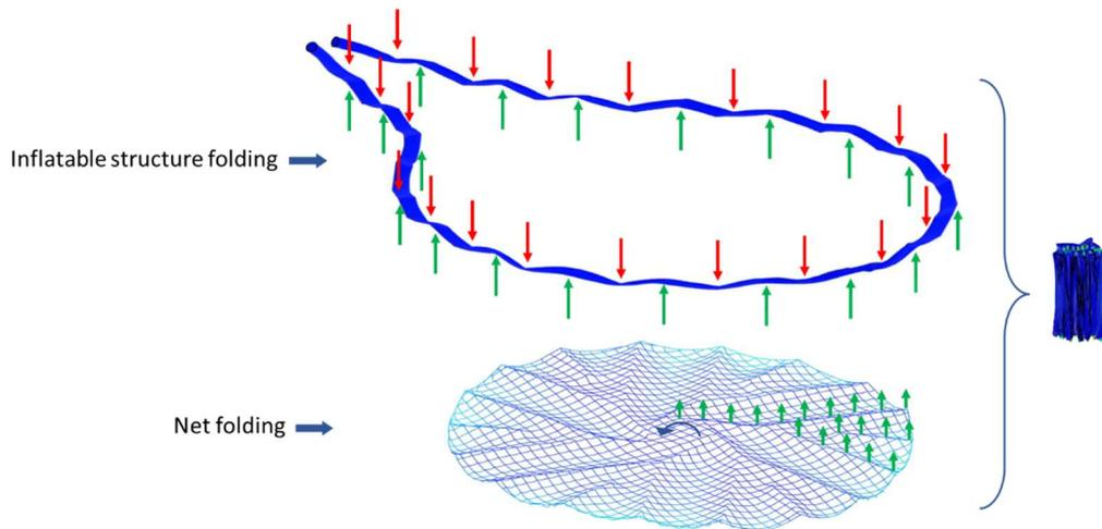
Figure 8: Folding schemes of the inflatable structure and the net
