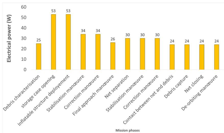
Figure 15 : INSIDeR kit power consumption according to the capture mission phases
