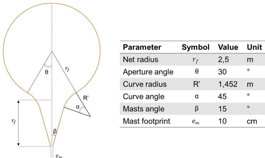
Figure 5: Geometrical shape of the inflatable structure
