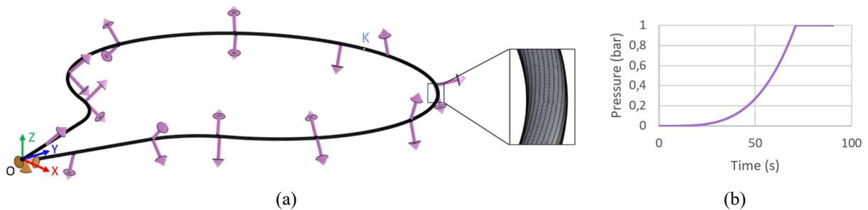
Figure 9: Finite element model of the inflatable structure
