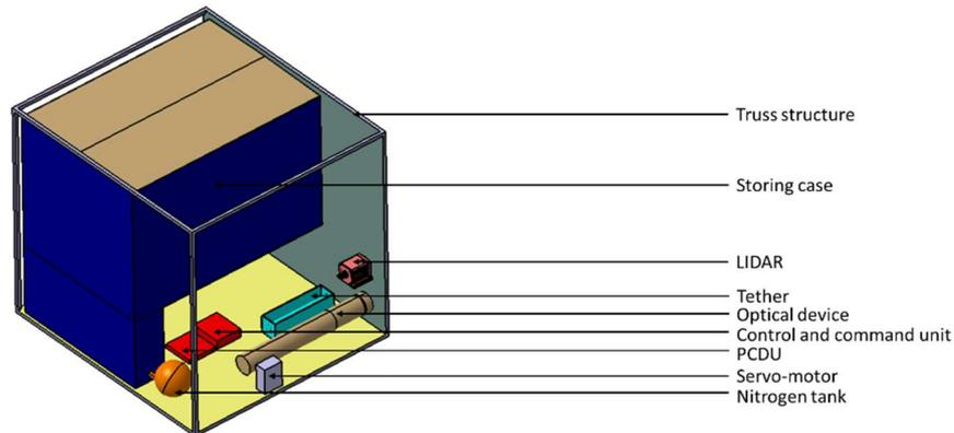
Figure 14: INSIDeR kit schematic
