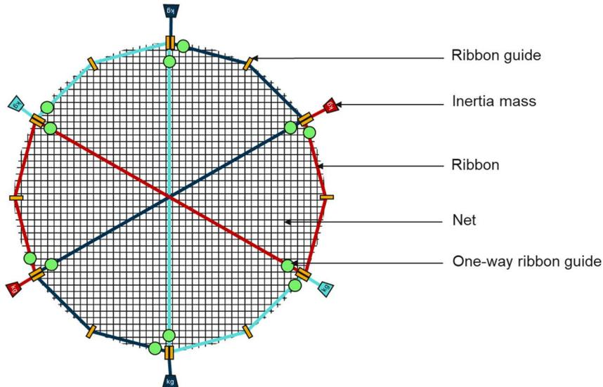
Figure 1: Net closing mechanism schematic
