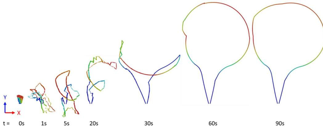
Figure 10: Deployment kinematics of the inflatable structure in the XY coordinates
