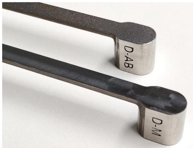
Figure 3: Channel floor sections (AB: as built; M: machined)
