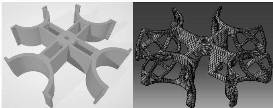
Figure 8 – Turbines plateau before (left) and after (right) its topological optimisation.
