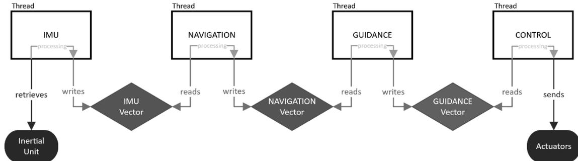
Figure 4 – Flight Software block diagram (within the main thread)
