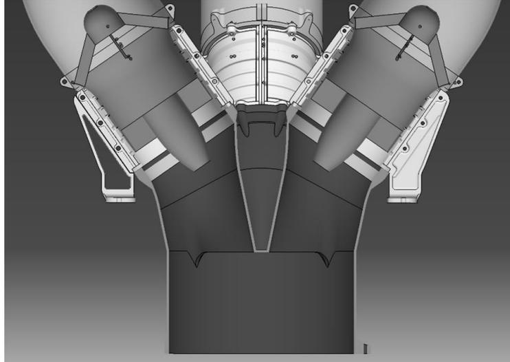
**Figure 3 - Sectional view of the airflow merger**
