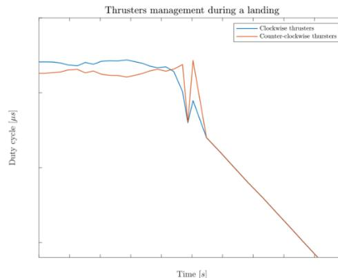
Figure 5 – Thrusters management during a landing sequence
