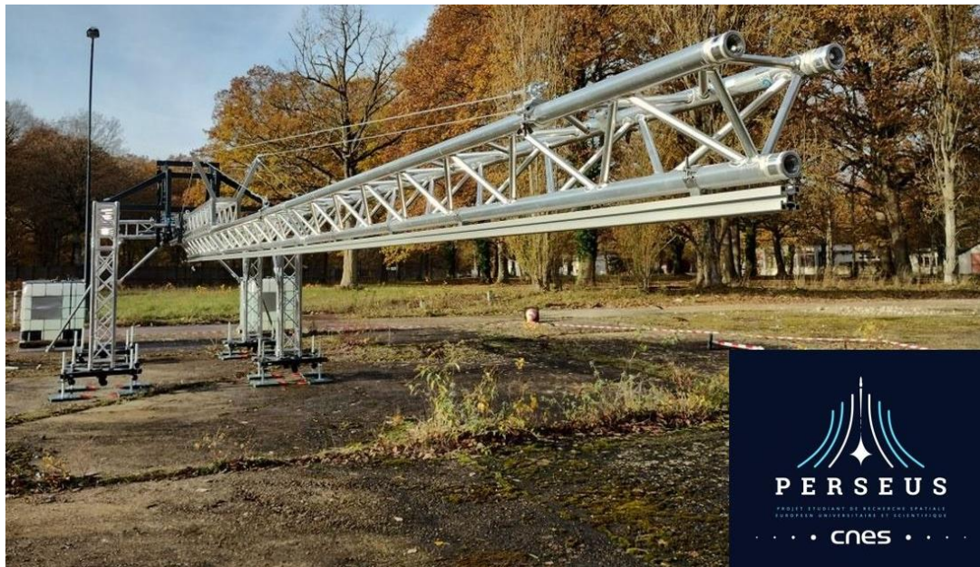
Figure 6 - View of the mobile launch rail in VERNON at the horizontal
