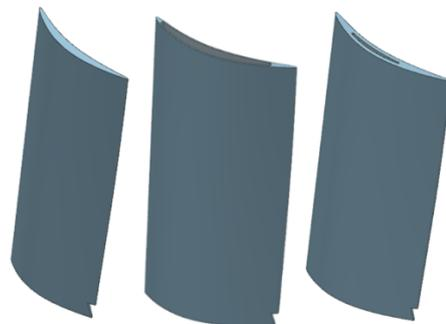
*Parameters:* Outer Case Forward and aft Stiffness Rib Height, Outer Case Thickness.
