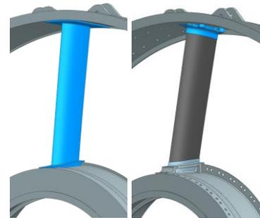
*Parameters:* Vane max thickness, Vane wall thickness, vane hollowness.
