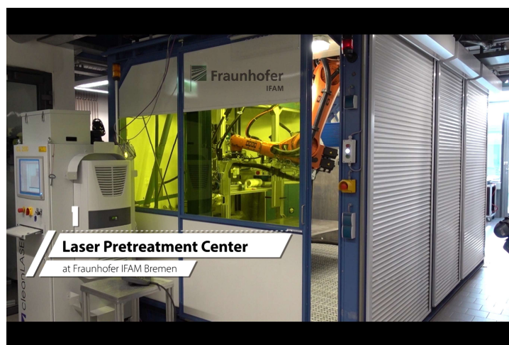
Figure 5: Facility for laser pretreatment of large, complex curved structures at Fraunhofer IFAM.
