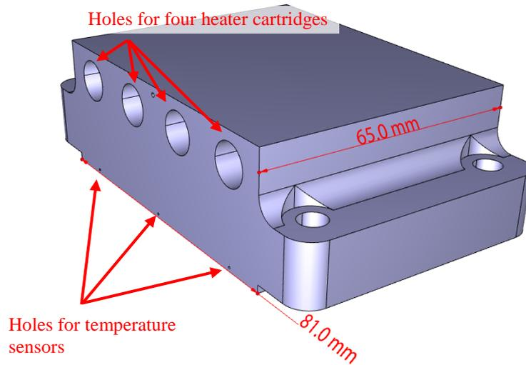
Figure 13: CAD drawing of a heater block that emulates the heat dissipation of a power module.
