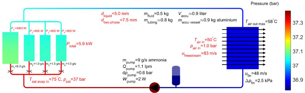
Figure 9: Calculated pressure with ammonia.
