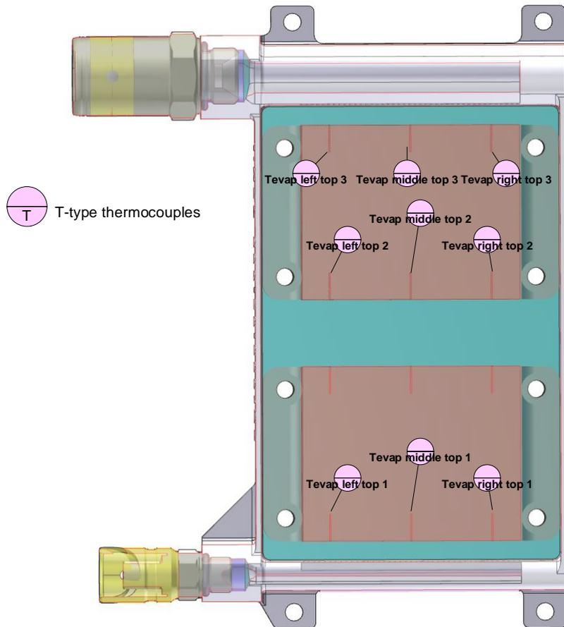
Figure 24: Cross-section with the location and name of the temperature sensors. There are 9 sensors on the top side of the coldplate (shown in figure) and 9 sensors on the corresponding location on the bottom side.
