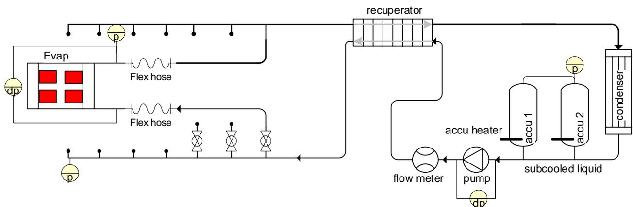
Figure 20: Schematic drawing of the test setup.
