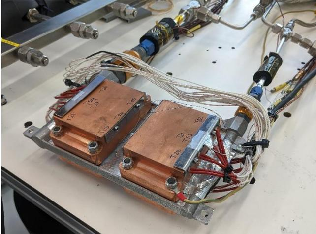
Figure 21: Photo of the evaporator plate in horizontal position without thermal insulation.
