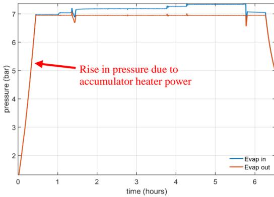
Figure 27: Measured absolute pressure.
