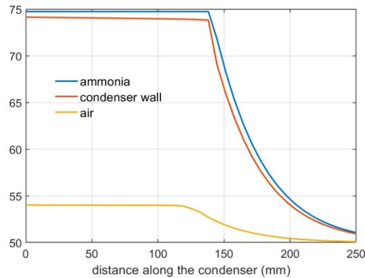
Figure 10: Calculated temperatures along the condenser, as indicated by the grey dashed line in Figure 7.
