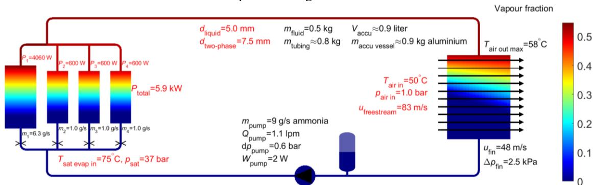
Figure 8: Calculated vapour mass fraction with ammonia.
