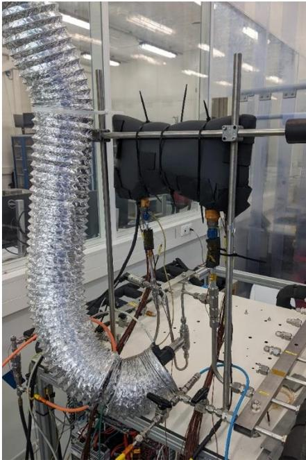
Figure 23: Photo of the evaporator plate in vertical position with thermal insulation.
