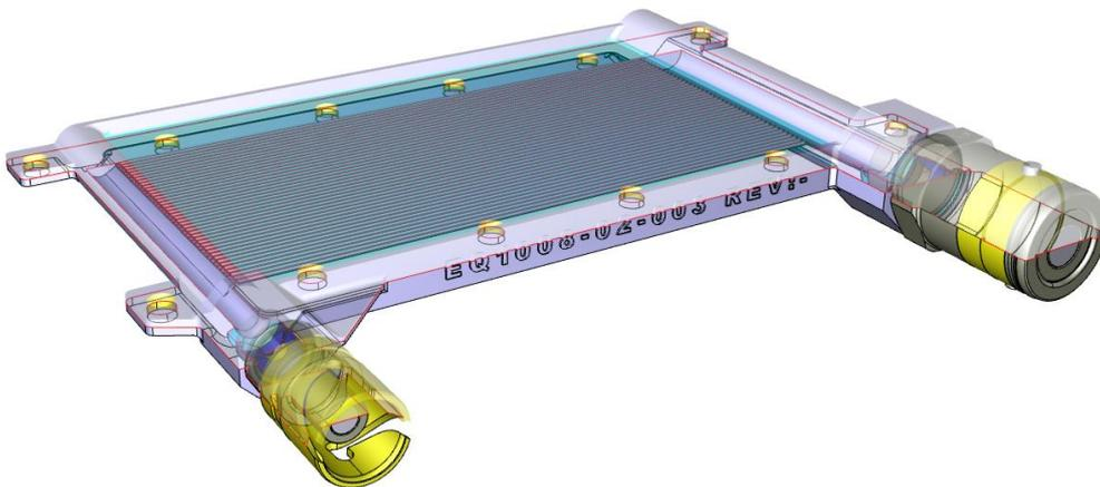
Figure 14: Cross section of the coldplate.
