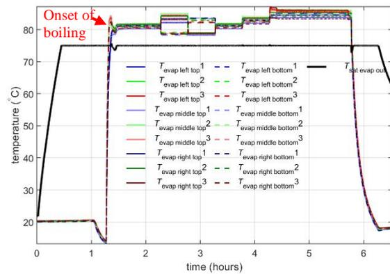
Figure 30: Measured temperatures on the evaporator plate.
