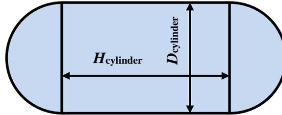
Figure 12: Schematic drawing of an accumulator vessel.
