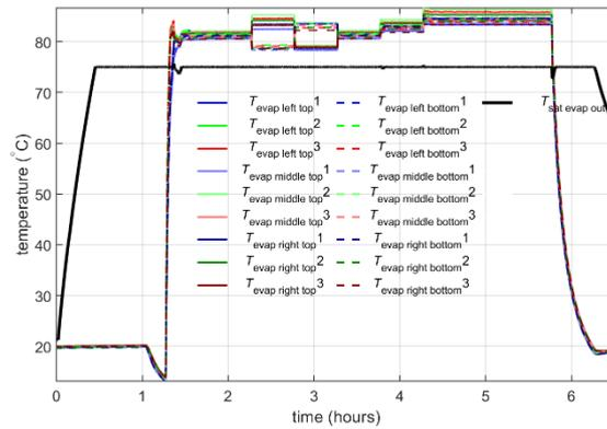
Figure 31: Measured temperatures on the evaporator plate in vertical orientation
