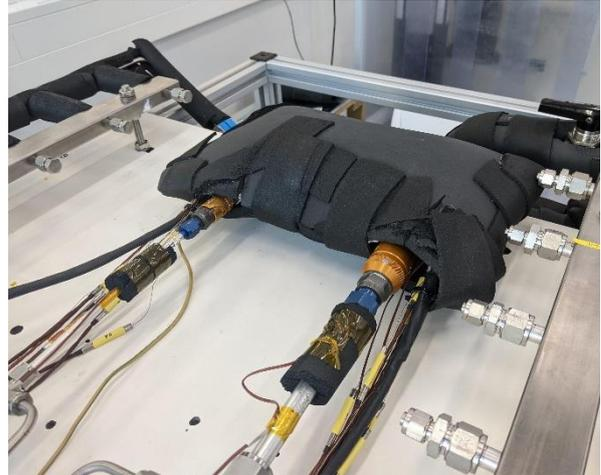
Figure 22: Photo of the evaporator plate in horizontal position with thermal insulation.
