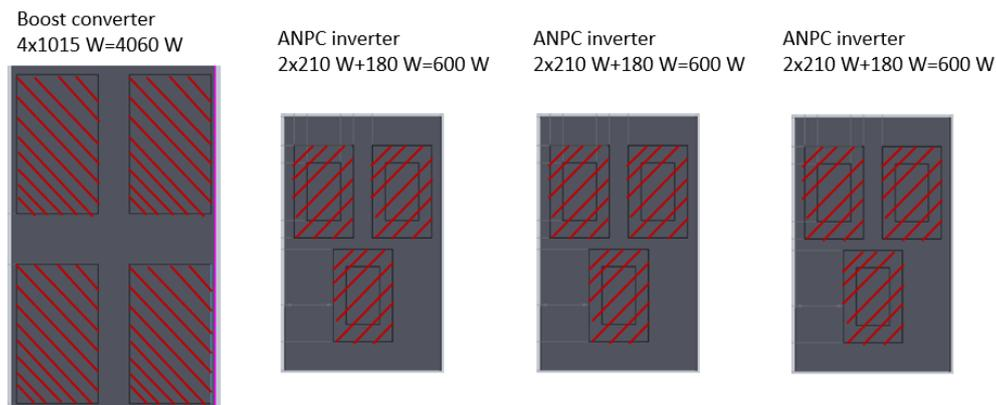
Figure 2: Schematic drawing of the four coldplates for the power electronics module for a single motor. The total amount of waste heat for the power electronics is  $4060 \text{ W} + 3 \times 600 \text{ W} = 5860 \text{ W}$ .
