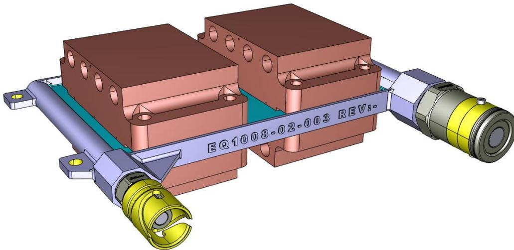
Figure 15: Coldplate with four heater blocks that emulate the heat dissipation of four power modules.
