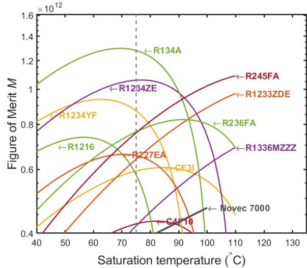
Figure 6: Figure of Merit for all fluids in the REFPROP database with a NFPA rating of 2 or lower.
