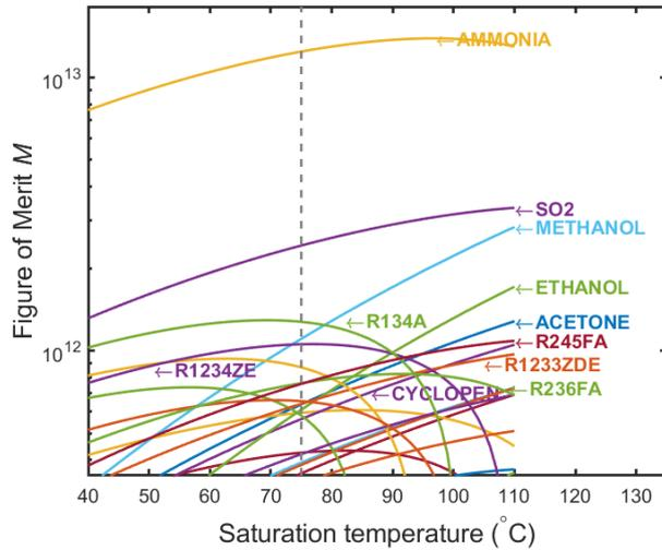
Figure 5: Figure of Merit for all fluids in the REFPROP database with a NFPA rating of 3 or lower.
