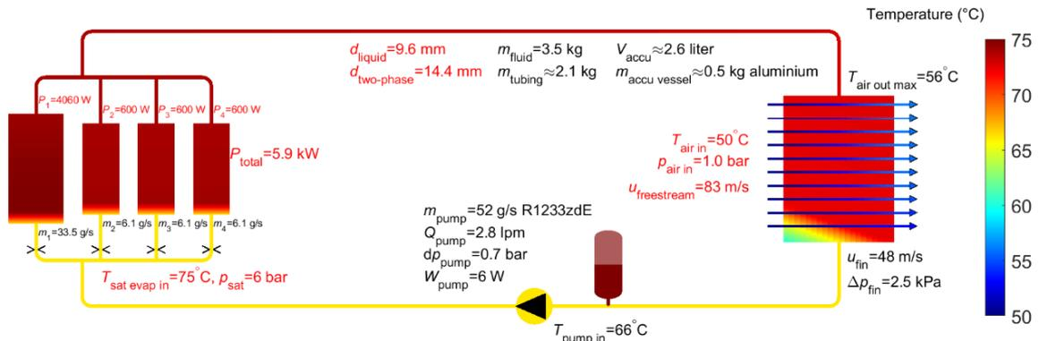
Figure 11: Calculated temperatures with R1233zd(E).
