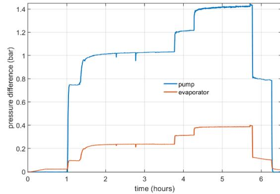
Figure 28: Measured pressure difference over the pump and evaporator.
