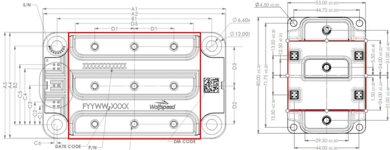
Figure 3: Drawing of a power module for a boost converter (left) and for an ANPC inverter (right). The waste heat is primarily generated within the rectangle indicate with the red line, which has an area of  $8.1 \text{ cm} \times 6.5 \text{ cm} = 52.65 \text{ cm}^2$  for the boost converter (resulting in a heat flux of  $19.3 \text{ W/cm}^2$ ) and  $4.8 \text{ cm} \times 5.3 \text{ cm} = 25.44 \text{ cm}^2$  for the ANPC inverter (resulting in a heat flux of  $8.3 \text{ W/cm}^2$ ).
