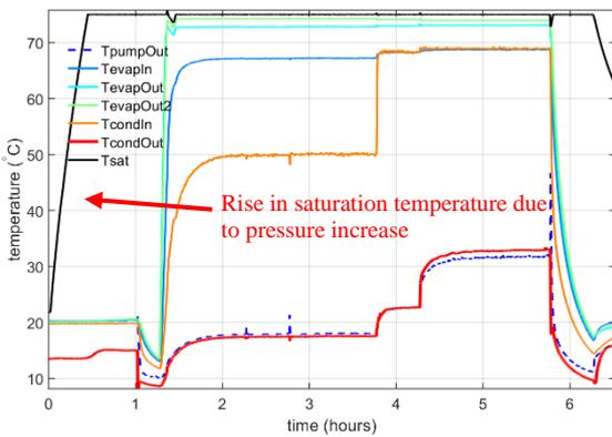
Figure 29: Measured temperatures at several locations.
