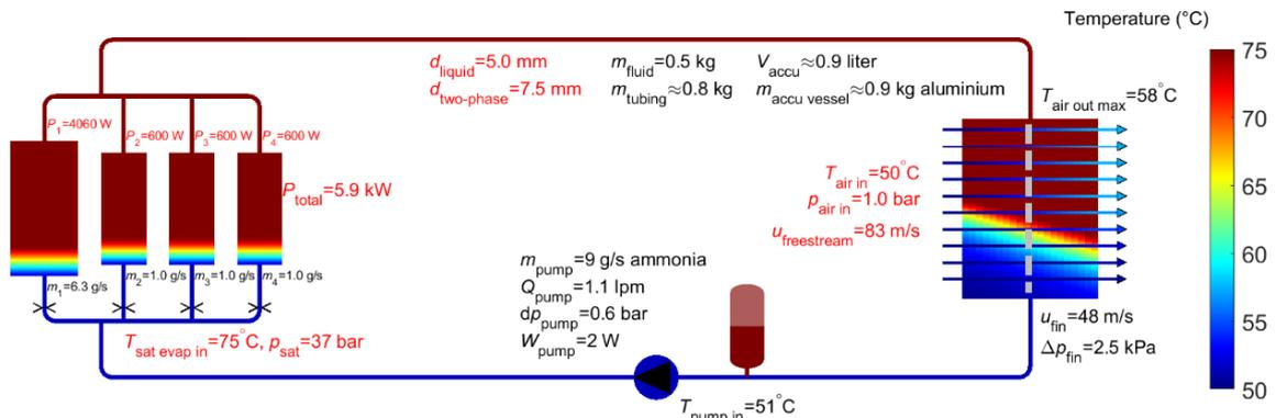
Figure 7: Calculated temperatures with ammonia. The temperature along the dashed grey line in the condenser is plotted in Figure 10.
