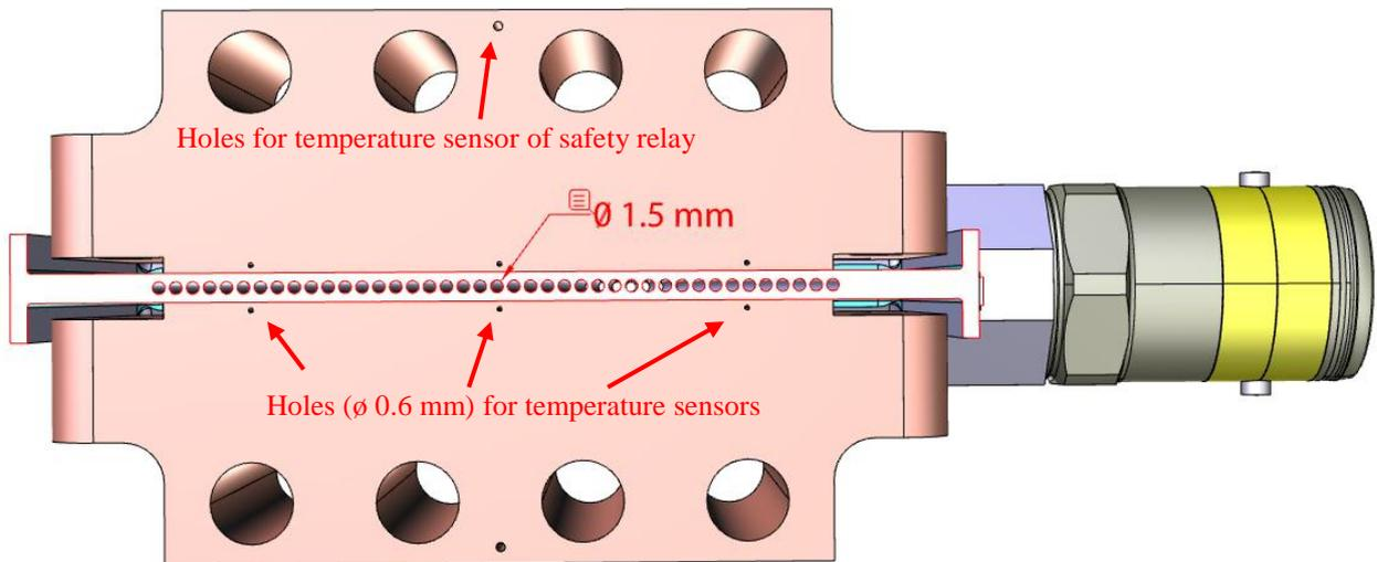
Figure 16: Cross-section of the evaporator plate with heater blocks mounted on both sides.
