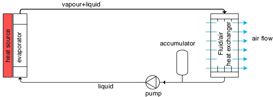
Figure 1: Schematic drawing of a two-phase MPL. The schematic of a liquid MPL is very similar, except that the fluid is in the liquid phase in the entire system.
