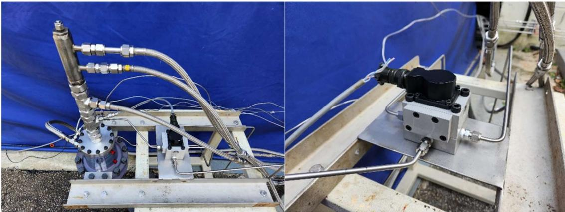
Figure 5: Installation of the pintle injector and hydraulic line at test stand
