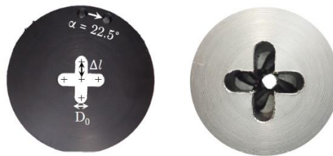
Figure 5: Port design of STEPHHY X [14]
