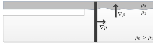
Figure 1: Interaction between longitudinal pressure gradient and radial density gradient in a typical shear coaxial injector. Image credit: [7].
