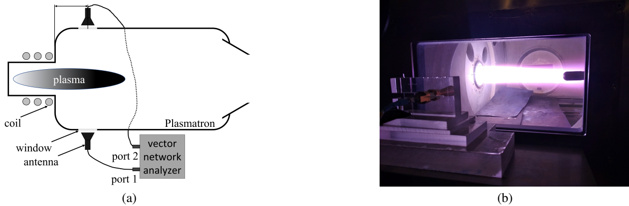
Figure 10: Schematic of the antenna positions with respect to the CFD domain (a) and a photograph with one of the antennas during a test in the Plasmatron (b). 26
