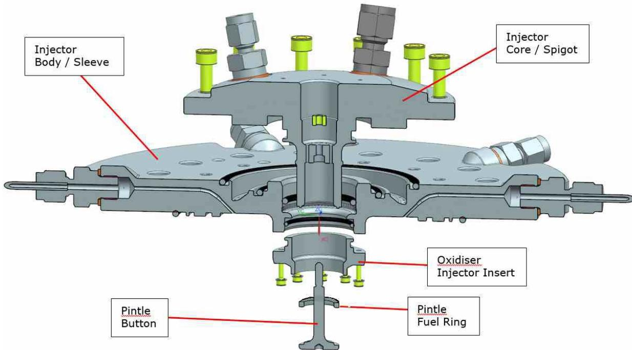
Figure 4: Exploded View of the Injector Assembly
