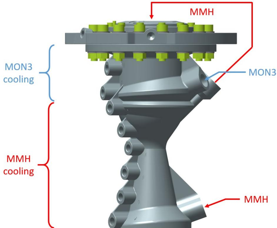
Figure 3: View of the Breadboard Engine without Tubing or Instrumentation
