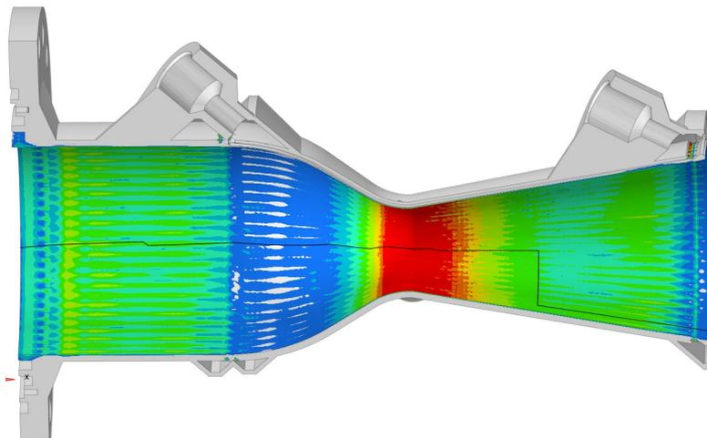
Figure 6: Strain along the Combustion chamber after Structural Analysis
