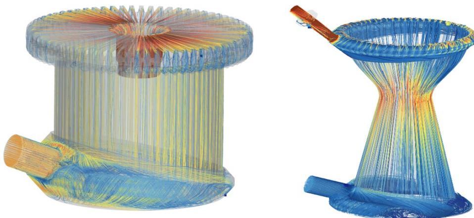
Figure 7: Velocity fields from CFD Analysis in MON-3 (Left) and MMH (Right) Cooling Jackets
