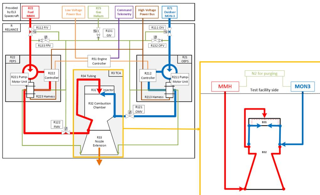
Figure 1: Breadboard Engine Schematic (right) Extracted from RELIANCE Engine Schematic (left)
