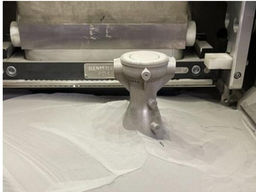
Figure 9: Remaining Powder after a Chamber Print
