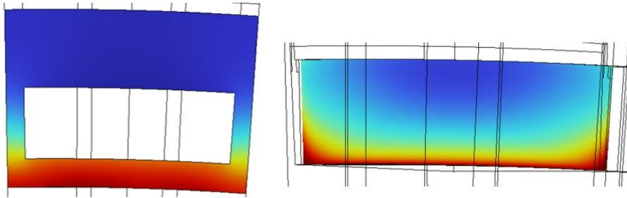
Figure 5: Wall (Left) and Propellant (Right) Temperatures in a Cooling Channel Section after Thermal Analysis
