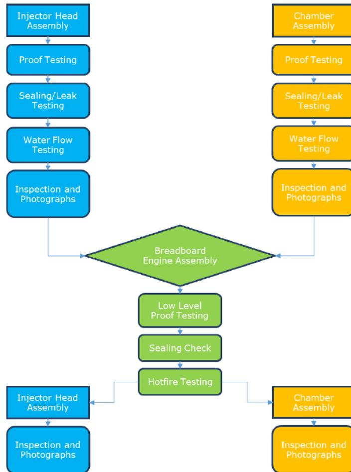
Figure 11: RELIANCE Breadboard Engine Test Flow
